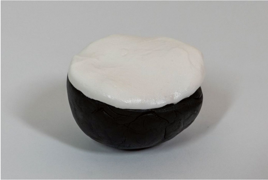
Figure 2-3. Black dough semicircle with a white insulating dough pancake on top
