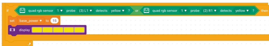
Figure 3-28. The duplicated block cluster from the green “if” block, with some values changed so it can be applied to yellow tape
