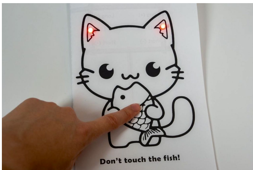
Figure 2-35. The finished project where pressing down on the battery behind the fish makes the two LEDs light up
