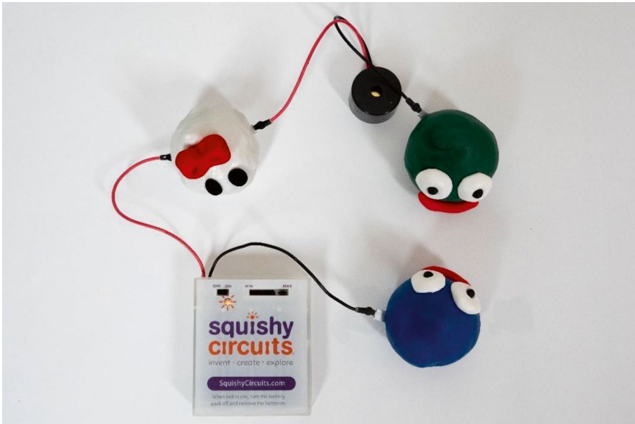
Figure 2-20. The wiring to connect all three slimes with the buzzer
