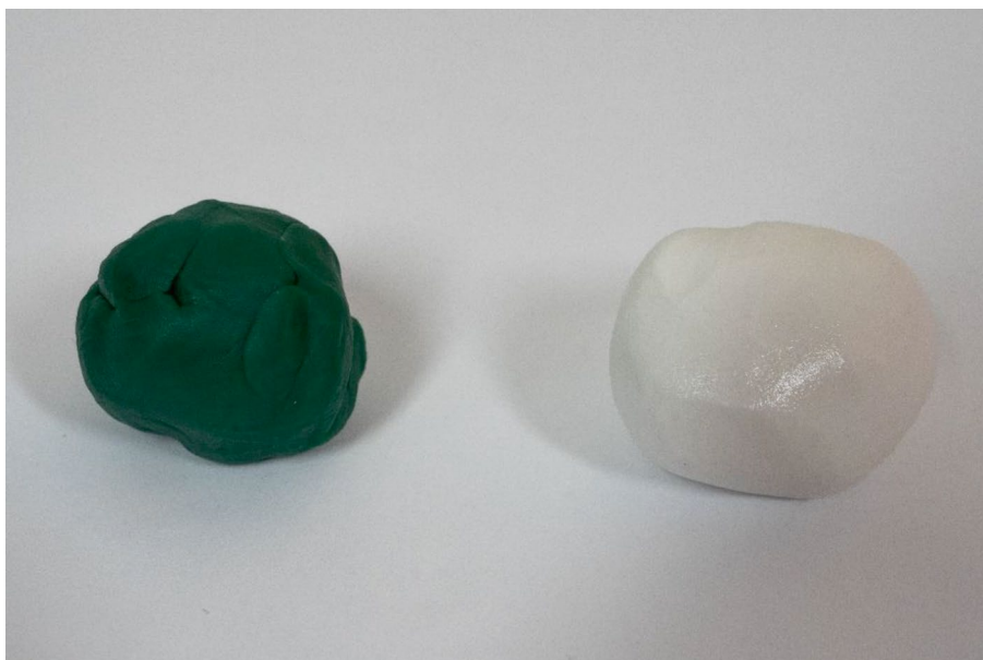
Figure 2-14. A colored play dough ball on the left and a slightly larger white insulating dough ball on the right
