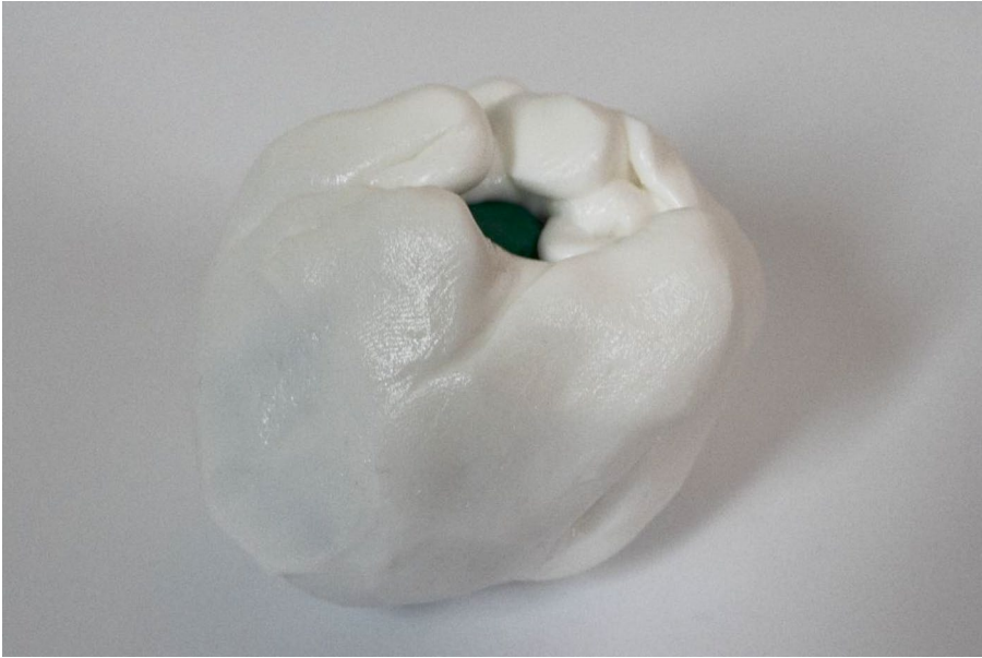
Figure 2-16. The white insulating dough wrapped around the colored conductive dough
