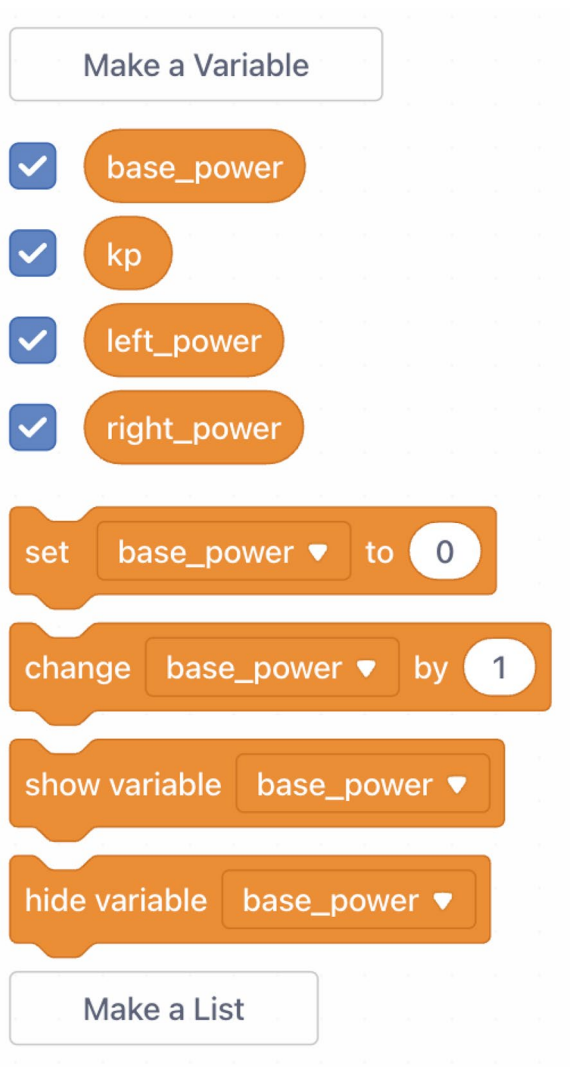
Figure 3-14. Creating four variables for the line follower robot
