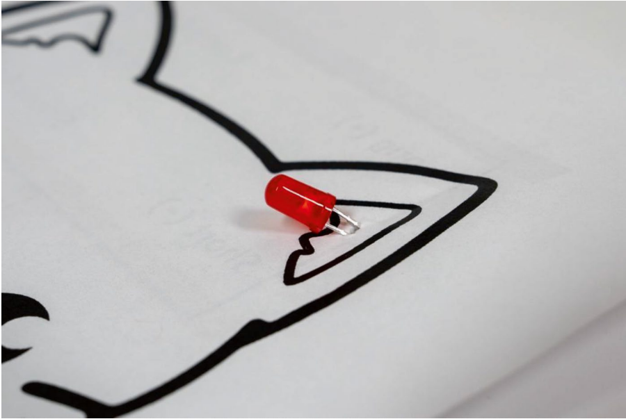
Figure 2-30. The LED light is used to poke a hole through the cat's ear
