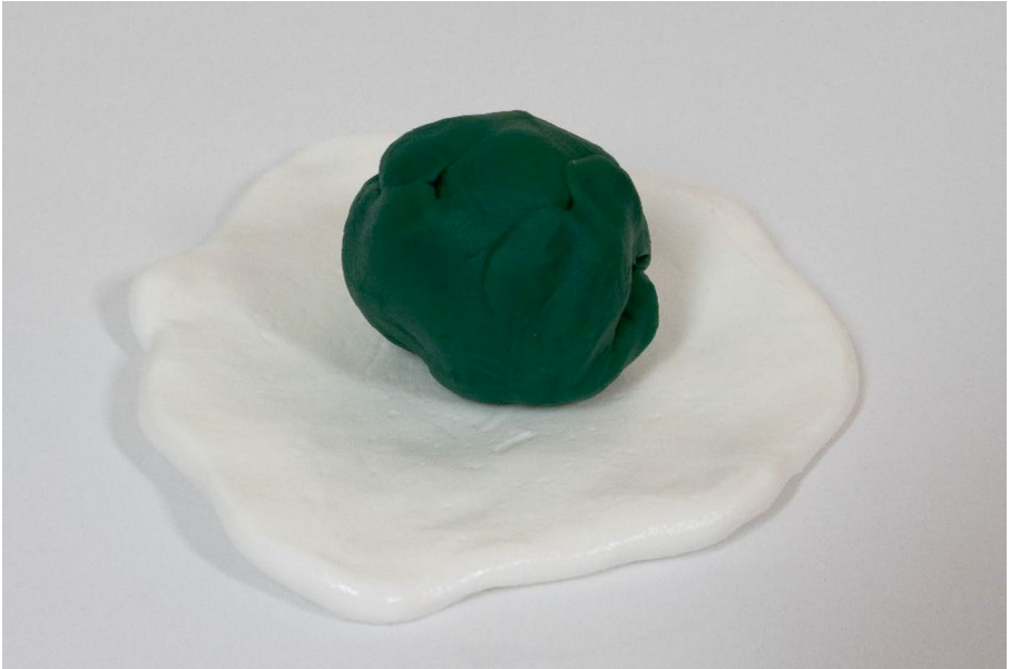
Figure 2-15. The white insulating dough is flattened into a pancake with the colored dough sitting in the center
