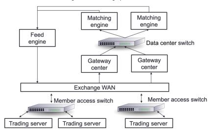
Figure 5.8 - Trading network infrastructure of trading exchange and trading servers
