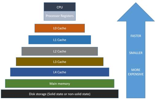
Figure 6.3 – Memory hierarchy in a modern architecture
