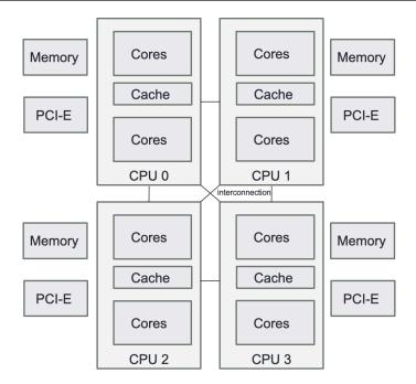
Figure 4.2 – A four-way NUMA architecture. Note how the CPUs form a fully connected graph in this configuration
