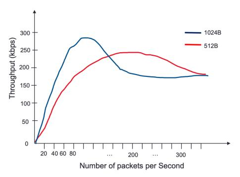
Figure 5.5 – Throughputs versus packet rate for different packet sizes
