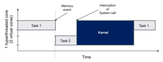
Figure 4.3 – Hyper-threading
