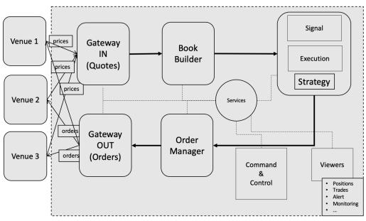
Figure 2.1 – Trading system architecture design
