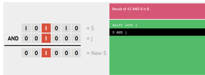
Figure 2.3: Bitmask Visualization, Example of CheckBit(j) Operation
