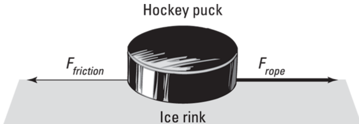
FIGURE 5-6: Pulling a heavy puck with a rope to overcome friction.
