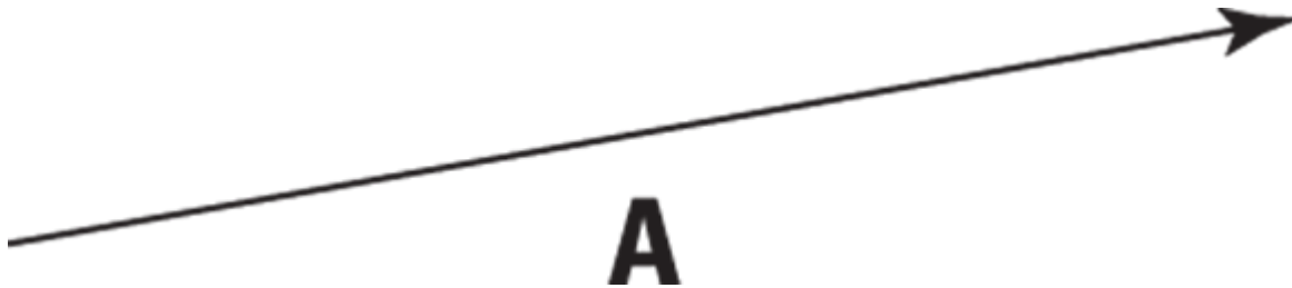
FIGURE 4-1: A vector, represented by an arrow, has both a direction and a magnitude.
