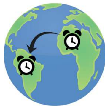
Fig. 2.3 Poincaré recognised that the concept of simultaneity must depend on the rule of clock synchronisation. Two clocks at distant locations can be synchronised only by accounting for the propagation time of a signal from one clock to another.
