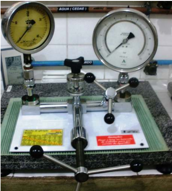
Fig. 5.4 Calibration of a pressure gauge. (Photo by the authors)
