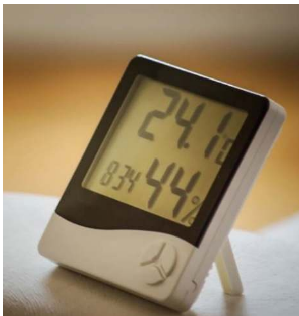
Fig. 2.11 Digital thermohygrometer (temperature and relative humidity). ( https://pixabay.com/photos/time-clock-humidity-air-hygrometer-2353382/ )
