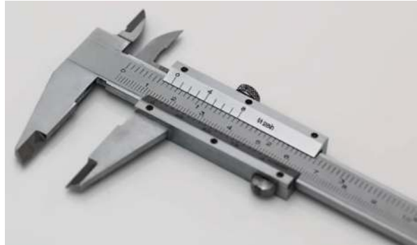
Fig. 2.12 Vernier caliper. ( https://pixabay.com/photos/vernier-caliper-measuring-instrument-452987/ )
