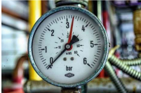
Fig. 2.15 Bourdon gauge. ( https://pixabay.com/photos/pressure-manometer-measure-up-1646350/ )
