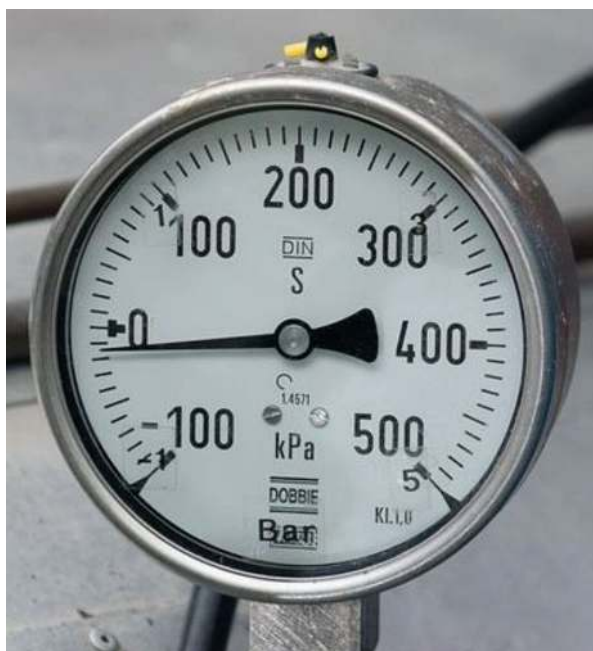
Fig. 4.6 Manometer: vacuum and positive pressure. ( https://pixabay.com/photos/pressure-meter-engineering-gauge-2113401/ )
