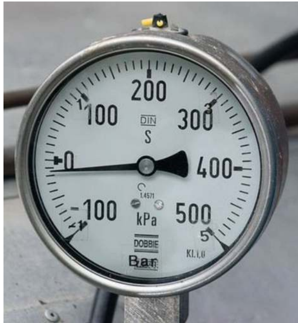
Fig. 4.8 Manometer with division of scale equal to 10 kPa and resolution of 5 kPa. ( https://pixabay.com/photos/pressure-meter-engineering-gauge-2113401/ )
