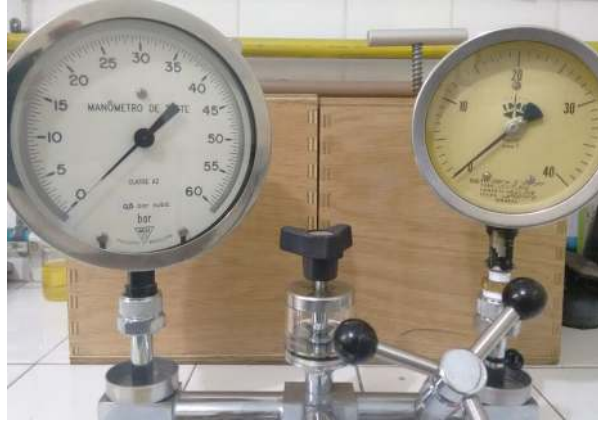
Fig. 3.4 Pressure gauge calibration. (Photo by the authors)
