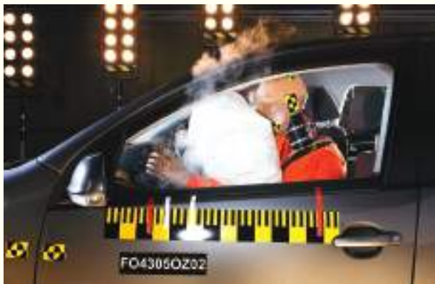
In a head-on collision, the air bag inflates rapidly to prevent the rider from moving forward and colliding with the windshield or steering column. fStop Images GmbH/Alamy Stock Photo
