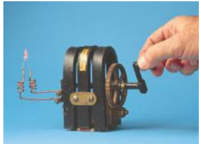
Figure 14.23 A simple generator consists of a coil of wire that generates an electric current when turned between the pole faces of permanent magnets. James Ballard/McGraw-Hill Education
