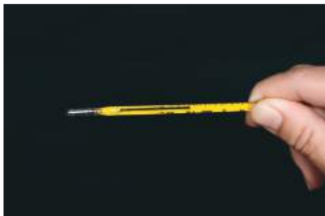
Figure 10.3 The traditional clinical thermometer contained mercury in a thin glass tube with a wider reservoir of mercury at the bottom.
