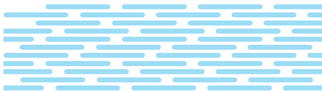
Figure 21.20 The long molecules in some liquid crystals line up in layers, allowing the liquid to flow along these layers but not in the perpendicular direction.
