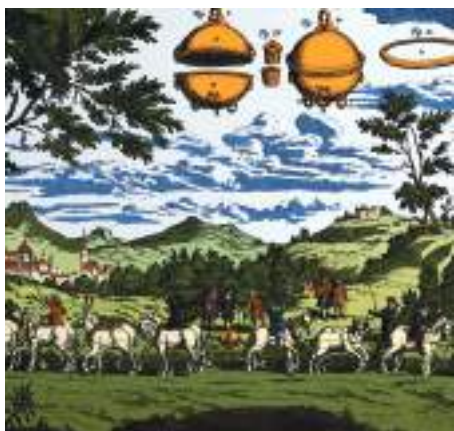
Figure 9.8 Two teams of eight horses were unable to separate the hemispheres of von Guericke's evacuated metal sphere. What force pushes the two hemispheres together? Colorization by: Robin Treadwell/Science Source
