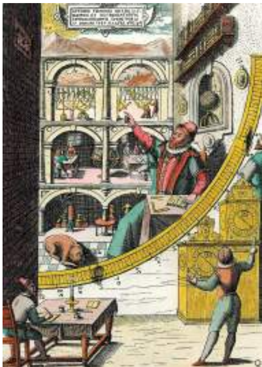
Figure 5.14 Tycho Brahe's large quadrant permitted accurate measurement of the positions of the planets and other heavenly bodies. Photo Josse/Leemage/Getty Images
