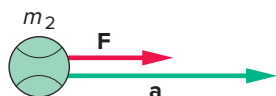
Figure 4.5 The smaller-mass object experiences a larger acceleration than the larger-mass object when identical forces are applied to the two objects.
