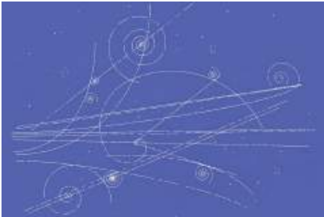
Figure 21.3 Particle tracks in a bubble chamber (or in modern electronic detectors) provide information on the new particles produced in collisions and decays. Zmeel Photography/E+/Getty Images
