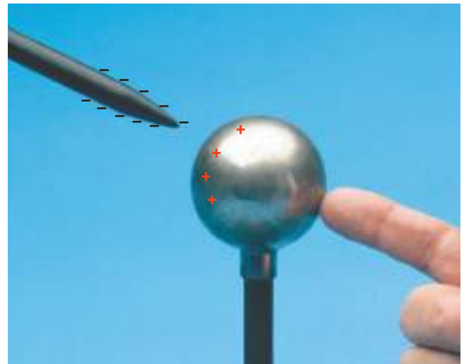
Figure 12.8 Touching a finger to the opposite side of the metal ball draws off the negative charge, leaving the ball with a net positive charge. James Ballard/McGraw-Hill Education
