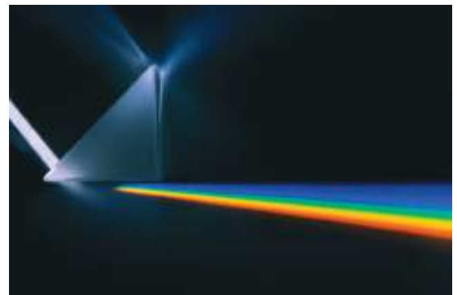
Figure 17.14 White light incident on one side of the prism emerges as a spectrum of different colors because of dispersion. Don Farrall/Getty Images
