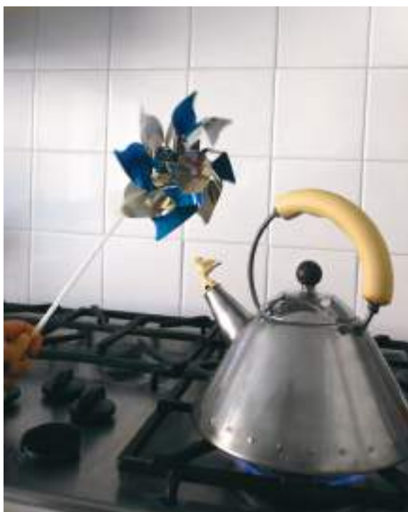
Figure 11.5 Steam issuing from the kettle makes the pinwheel turn in this simple steam turbine. Work could be done to lift a small weight with such an engine.
