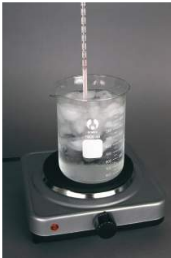
Figure 10.10 Adding heat to a mixture of water and ice at 0^\circ\text{C} melts the ice without changing the temperature of the mixture.
