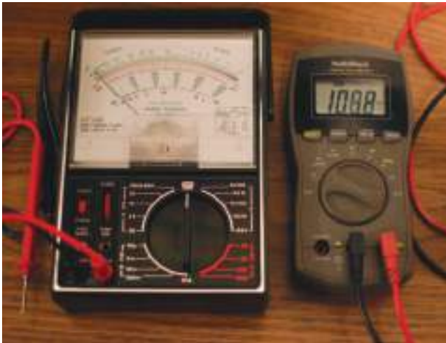
Figure 13.11 An analog multimeter (with needle and separate scales) and a digital multimeter are commonly used measuring instruments.
