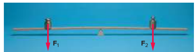
Figure 8.5 A simple balance with equal weights placed at equal distances from the fulcrum.
