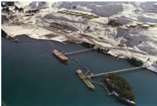
Figure 9.17 A fully loaded tanker rides much lower in the water than an empty tanker. Chris Wilkins/AFP/Getty Images
