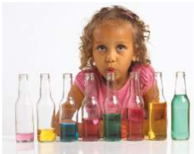
Figure 15.18 Placing your lower lip at the rim of a soft-drink bottle and blowing softly across the opening produces a standing wave in the bottle. Dave King/Dorling Kindersley/Getty Images
