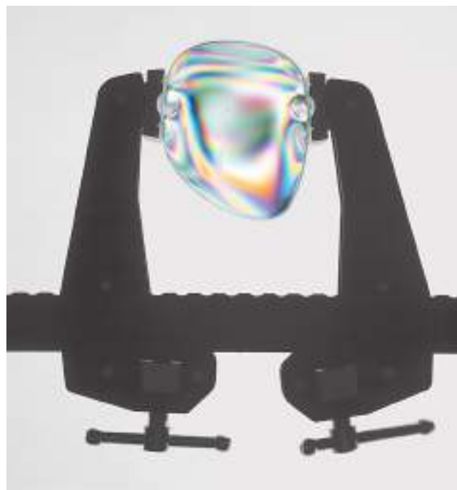
Figure 16.26 A plastic lens being compressed between two clamps shows stress birefringence when viewed between crossed polarizers. Diane Hirsch/Fundamental Photographs, NYC
