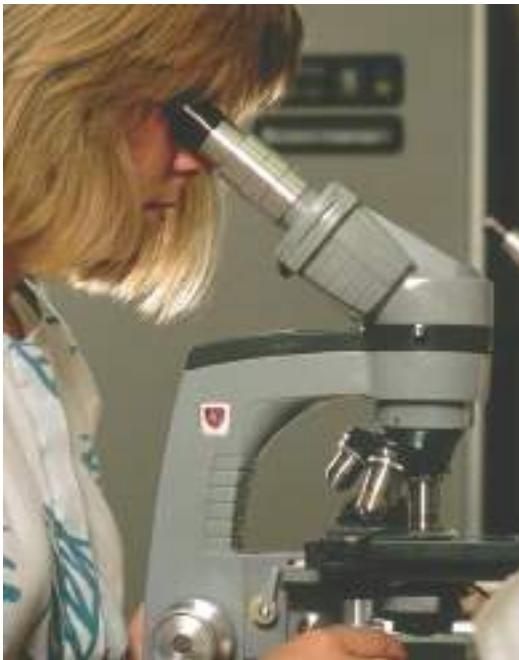
Figure 17.28 A laboratory microscope often has three or four objective lenses mounted on a rotatable turret. Light passes through the object slide from a source below the slide. James Ballard/McGraw-Hill Education
