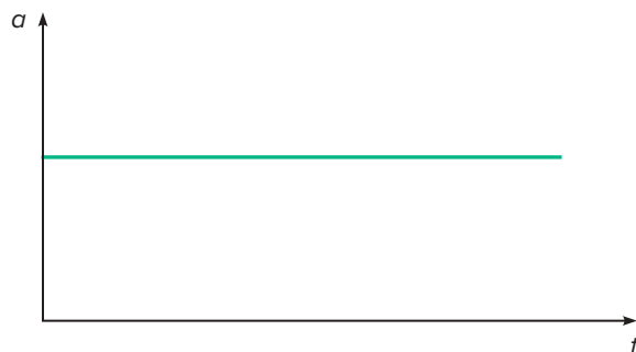
Figure 2.17 The acceleration graph for uniform acceleration is a horizontal line. The acceleration does not change with time.
