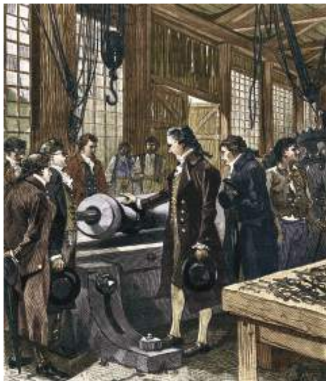
Figure 10.11 Rumford's cannon-drilling apparatus. What is the source of heat that raises the temperature of the drill and the cannon barrel?
