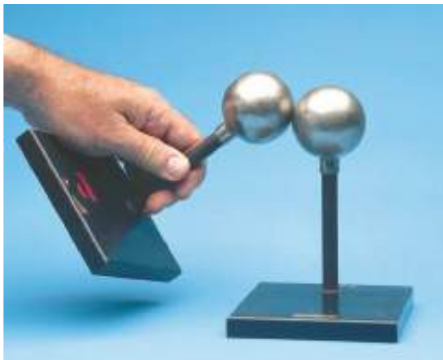
Figure 12.12 By bringing two identical metal balls into contact, one charged and the other one initially uncharged, equal quantities of charge are obtained on the two balls. James Ballard/McGraw-Hill Education
