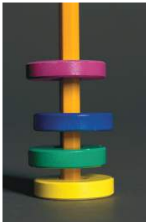
Figure 14.4 Ring magnets levitating on a vertical wooden rod. The rod keeps the magnets from flying off to the side. Lars A. Niki/McGraw-Hill Education
