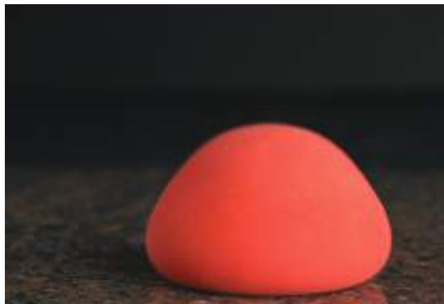
Figure 7.3 Two high-speed photographs of a ball hitting a tabletop, one just before the impact and the other after the impact. The ball is compressed like a spring. (both): Ted Kinsman/Science Source
