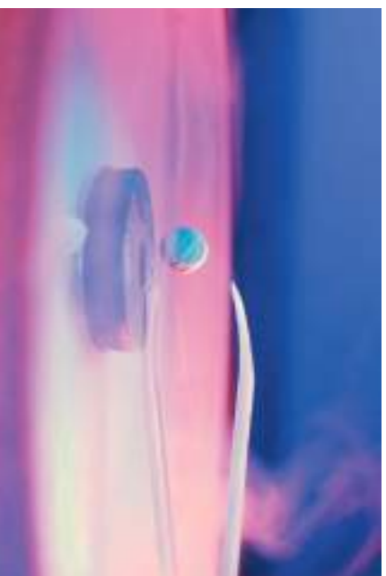
Figure 21.17 A small magnet levitates above a superconducting disk cooled with liquid nitrogen. This simple test establishes the presence of superconductivity.
