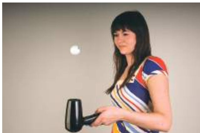
Figure 9.26 A ball is suspended in an upward-moving column of air produced by a hair dryer. The air pressure is smallest in the center of the column, where the air is moving with the greatest speed.
