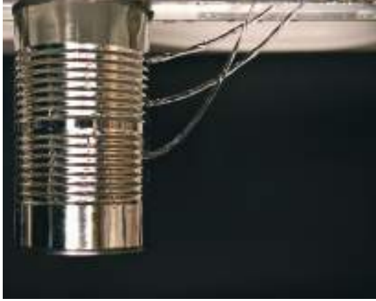
Figure 9.15 Water emerging from a hole near the bottom of a can filled with water has a larger horizontal velocity than water emerging from a hole near the top.
