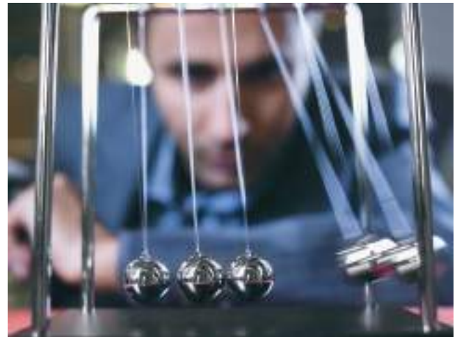
Figure 7.16 The swinging-ball apparatus provides an example of collisions that are approximately elastic. Mike Kemp/RubberBall/SuperStock
