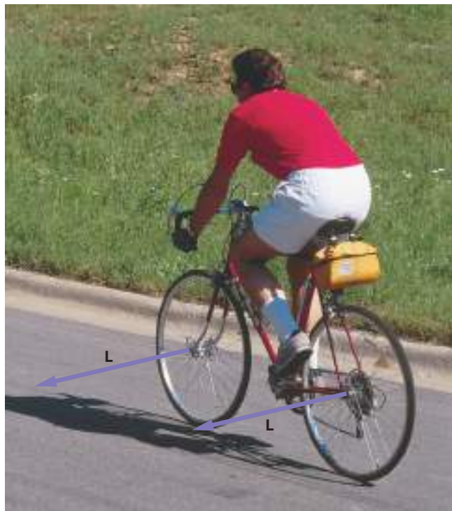
Figure 8.21 The angular-momentum vector for each wheel is horizontal when the bicycle is upright.
