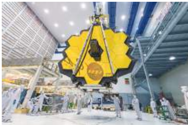
Figure 21.1 The James Webb Space Telescope will complement and extend the discoveries of the Hubble Space Telescope. The anticipated launch date is October 2021. In this photo, NASA technicians lift the mirror for the telescope using a crane and move it inside a clean room at NASA's Goddard Space Flight Center in Greenbelt, Maryland.
