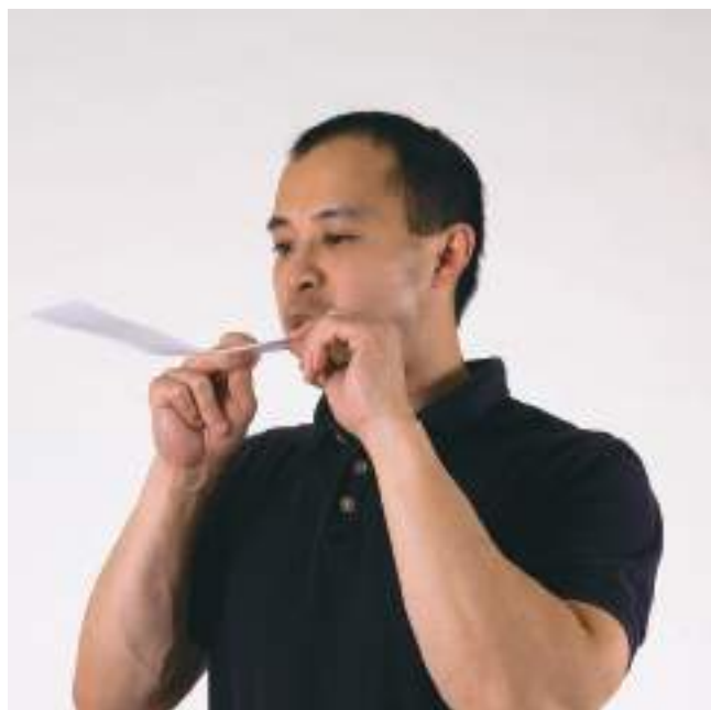
Figure 9.25 Blowing across the top of a limp piece of paper causes the paper to rise, demonstrating Bernoulli's principle. Jill Braaten/McGraw-Hill Education
