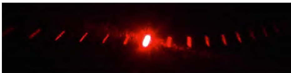
Figure 4.12 (a) Intensity of light transmitted through a large number of slits. When N approaches infinity, only the principal maxima remain as very bright and very narrow lines. (b) A laser beam passed through a diffraction grating. (credit b: modification of work by Sebastian Stapelberg)
