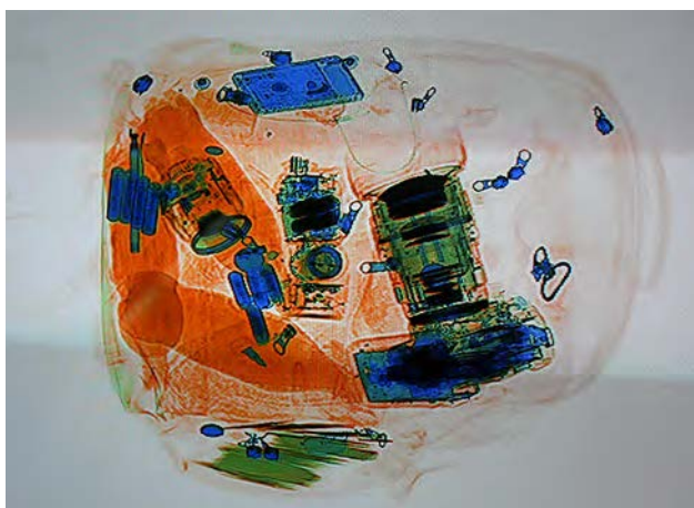
Figure 8.26 An X-ray image of a piece of luggage. The denser the material, the darker the shadow. Object colors relate to material composition—metallic objects show up as blue in this image. (credit: “IDuke”/Wikimedia Commons)
