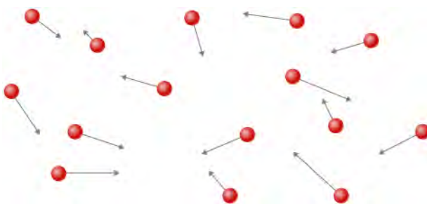
Figure 2.2 Atoms and molecules in a gas are typically widely separated. Because the forces between them are quite weak at these distances, the properties of a gas depend more on the number of atoms per unit volume and on temperature than on the type of atom.
