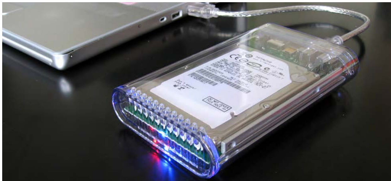
Figure 12.1 An external hard drive attached to a computer works by magnetically encoding information that can be stored or retrieved quickly. A key idea in the development of digital devices is the ability to produce and use magnetic fields in this way. (credit: modification of work by “Miss Karen”/Flickr)
