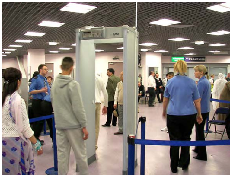
Figure 14.9 The familiar security gate at an airport not only detects metals, but can also indicate their approximate height above the floor. (credit: “Alexbuirds”/Wikimedia Commons)
