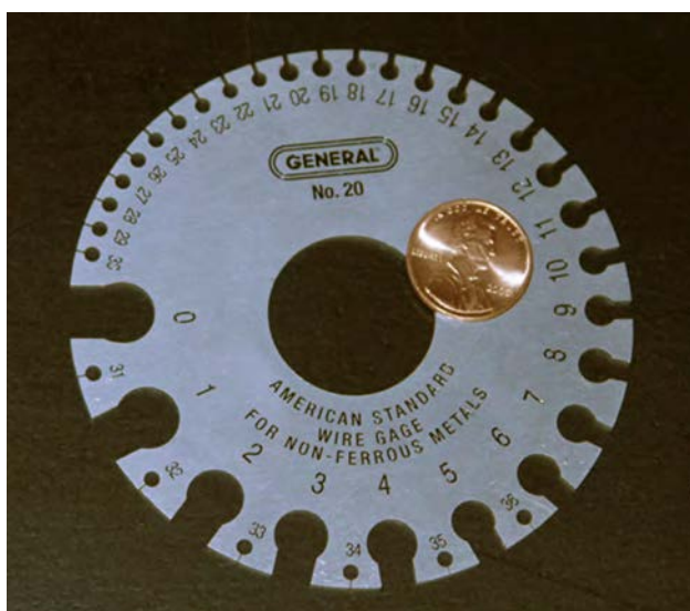
Figure 9.11 A device for measuring the gauge of electrical wire. As you can see, higher gauge numbers indicate thinner wires.
