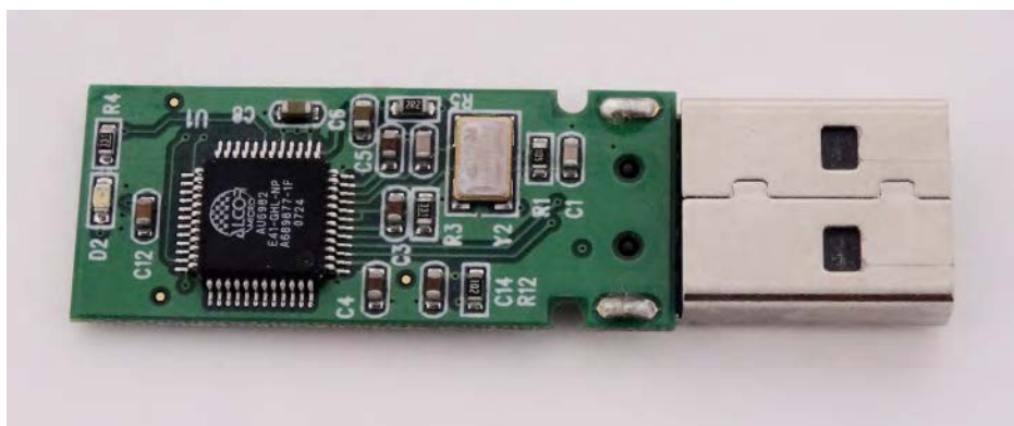
Figure 8.15 The capacitors on the circuit board for an electronic device follow a labeling convention that identifies each one with a code that begins with the letter “C.”
