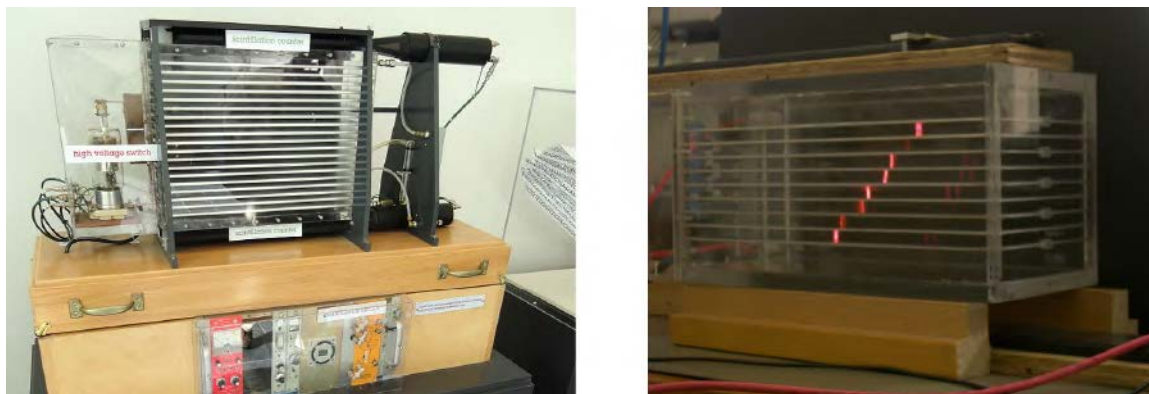
Figure 7.16 A spark chamber is used to trace the paths of high-energy particles. Ionization created by the particles as they pass through the gas between the plates allows a spark to jump. The sparks are perpendicular to the plates, following electric field lines between them. The potential difference between adjacent plates is not high enough to cause sparks without the ionization produced by particles from accelerator experiments (or cosmic rays). This form of detector is now archaic and no longer in use except for demonstration purposes. (credit b: modification of work by Jack Collins)
