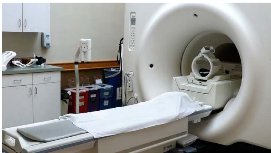
Figure 12.21 In an MRI machine, a large magnetic field is generated by the cylindrical solenoid surrounding the patient. (credit: Liz West)
