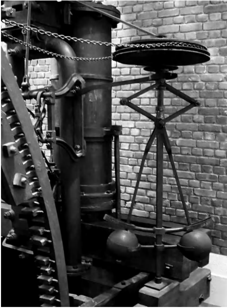
Figure 8.1: The governor mechanism of a Boulton and Watt steam engine of 1788 is a classic feedback system. The engine spins the mechanism and the two balls. Increasing speed means increasing centrifugal force, and that spreads the balls apart. In turn this mechanically produces feedback to the engine slowing it down, thus reducing the centrifugal force. In effect the separation of the two balls is governed by a limit cycle, see §7.8.2. Dr. Mirko Junge, Science Museum, London; photo by CC BY 3.0 Deed.
