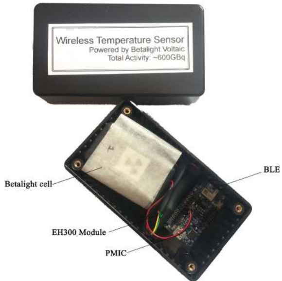
Fig. 6.1 Betalight-powered wireless sensor unit
