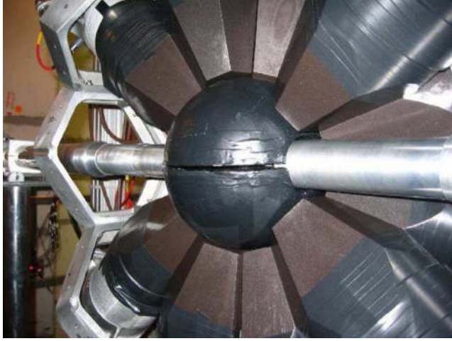
Figure 5.8. One hemisphere of the BaF 2 TAC array used in conjunction with nToF at CERN. Immediately surrounding the beampipe at the centre of the image is a neutron absorber shell. (Reproduced with permission from [18]. Copyright 2009 Elsevier.)
