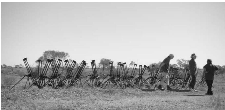
Rocket launchers left behind after the atomic testing at Maralinga. Hundreds of rockets were fired through each cloud immediately after detonation to take samples in the very first seconds of the chain reaction. (Courtesy of Daniel Everitt-Lock, True Perspective Films)
