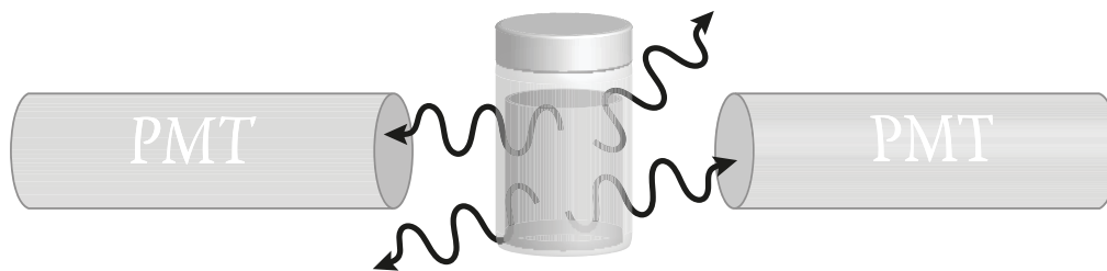
FIGURE 8.7 Organic scintillation gives off photons of visible light.
