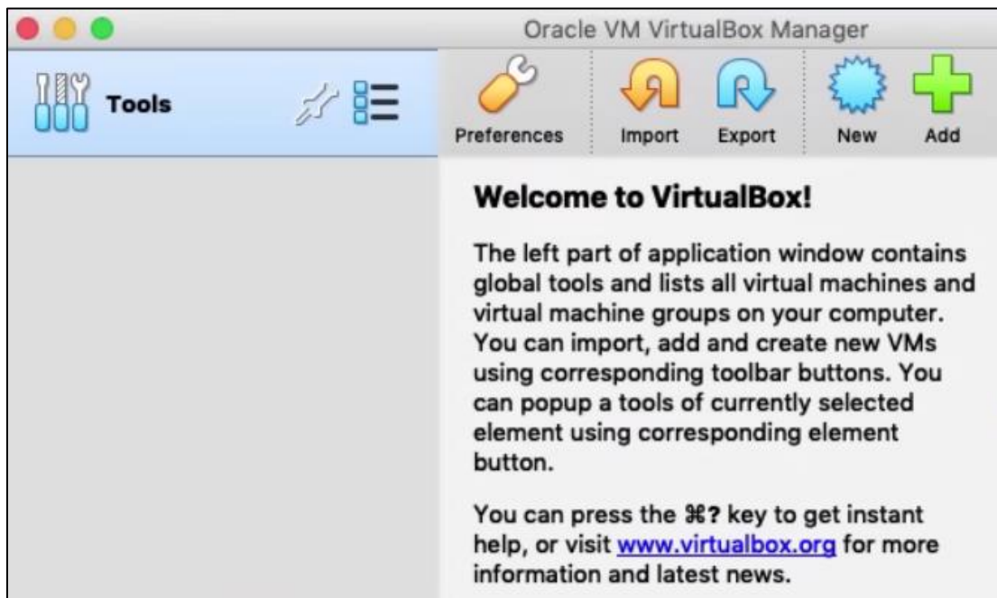
3-1: This is the graphical console for the hosted hypervisor, Oracle VirtualBox. This particular installation is running on top of MacOS. There are a host of icons along the top of the window (and various configuration menus) that allow the user modify various aspects of the hypervisor, and create virtual machines to suit their needs.
