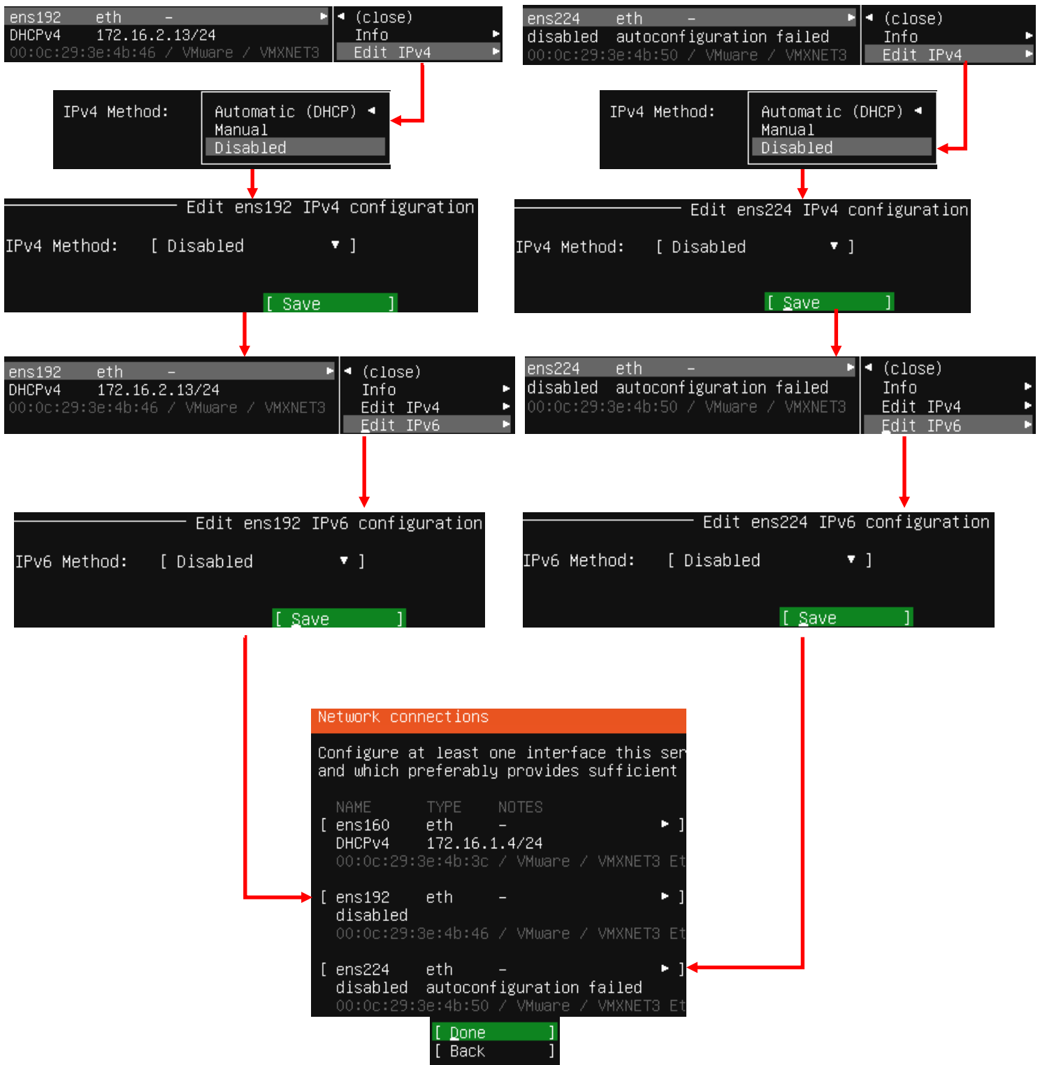
13-74: ens160 is the interface attached to the LAN network (Virtual Management port group), and should be the only interface with an IP address. Disable the other interfaces. They should never be assigned an IP address.
