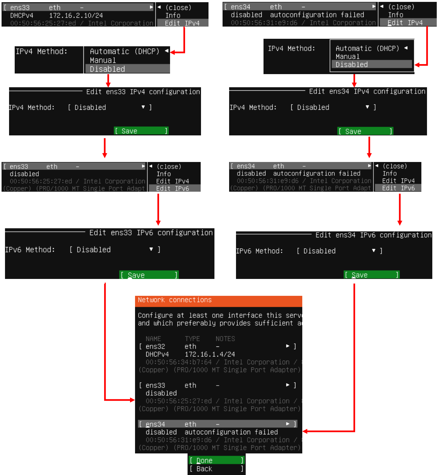
12-54: ens32 is the interface attached to the LAN network ( Host-only network), and should be the only interface with an IP address. Disable the other interfaces. They should never be assigned an IP address.
