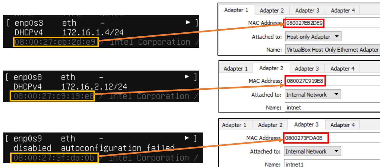
10-48: Ubuntu has assigned our three virtual adapters the interface names enp0s3, enp0s8, and enp0s9. Below each interface name is a MAC address. By cross referencing that MAC address to Adapter 1 , Adapter 2 , and Adapter 3 , we can determine which interface name maps to which virtual adapter, and confirm which network segment the interfaces are attached to. For instance, enp0s3 is adapter 1 , attached to the management/LAN network. enp0s8 is adapter 2 is attached to IPS 1/intnet, while enp0s9 is adapter 3 , attached to IPS 2/intnet1.
