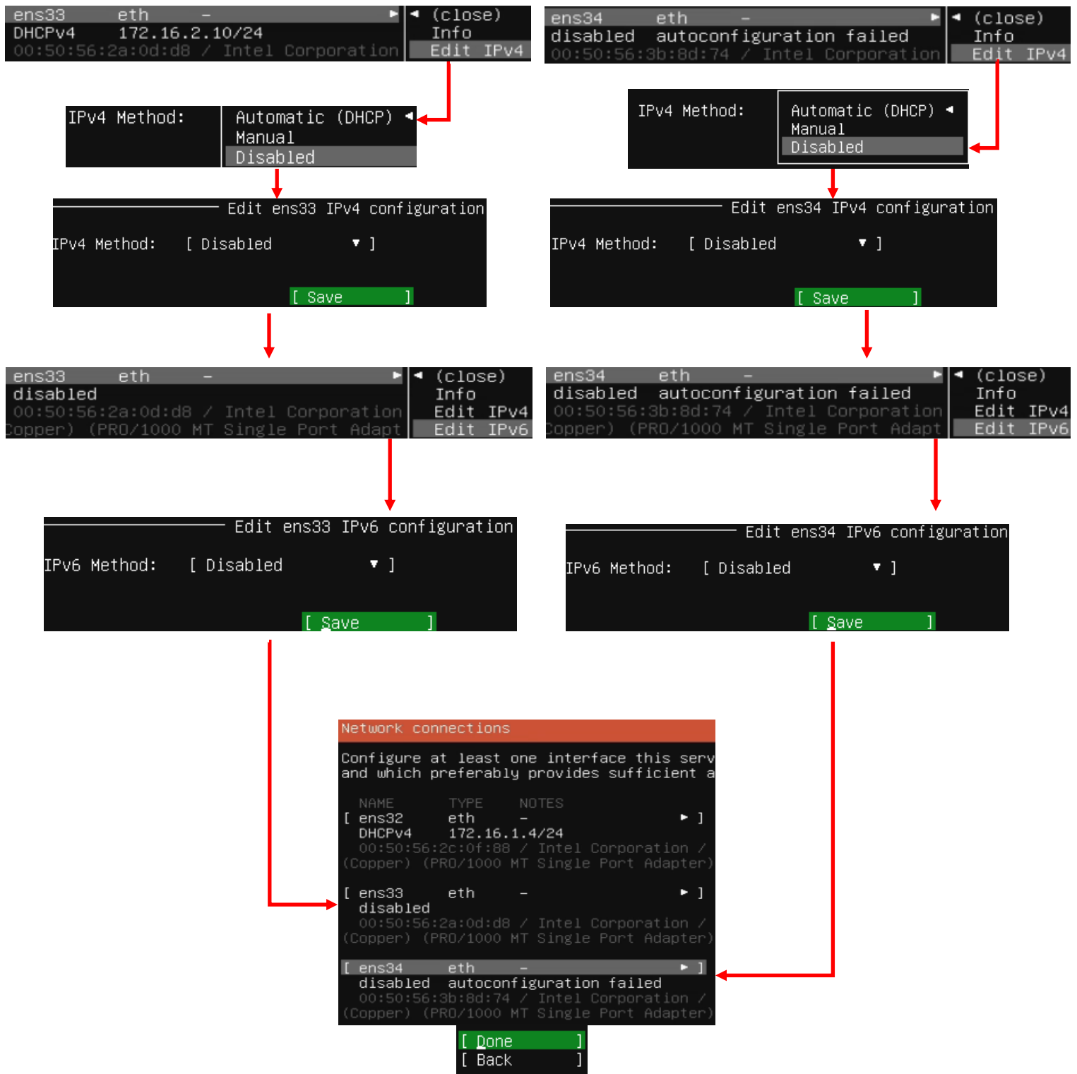
11-54: ens32 is the interface attached to the LAN network ( Host-only network), and should be the only interface with an IP address. Disable the other interfaces. They should never be assigned an IP address.
