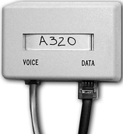
FIGURE 5-9 Properly labeled wall jack
