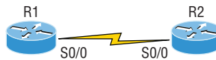
FIGURE 6.6 By looking at R1 using the show controllers command, you can see that R1 and R2 can't communicate.
