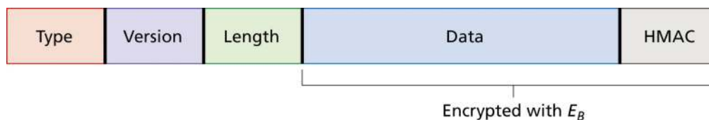
Figure 8.25: Record format for almost-TLS
