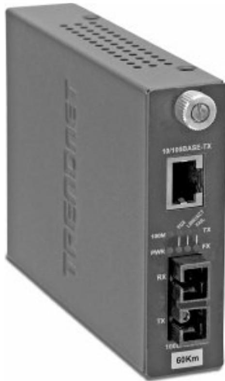
FIGURE 2.1-2 Typical copper-to-fiber Ethernet media converter (photo courtesy of TRENDnet)
