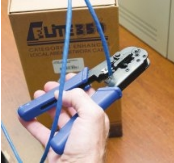
FIGURE 5.2-14 A crimper with built-in cable stripper
