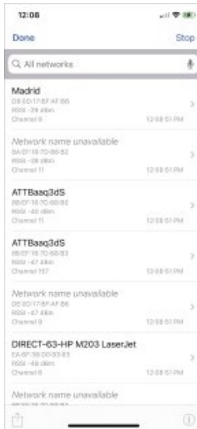
FIGURE 5.4-1 AirPort Utility showing RSSI strengths
