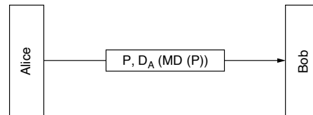
Figure 8-23. Digital signatures using message digests.
