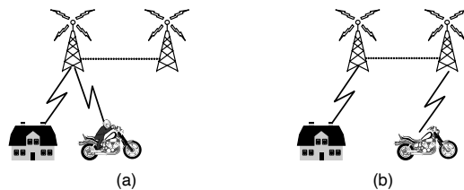
Figure 1-20. Mobile phone handover (a) before. (b) after.
