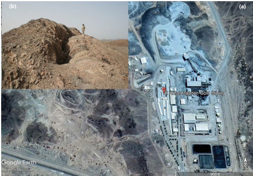
Fig 8.6 a Stellite image (via Google Maps) of the Al Amar gold mine site showing the carbon-in-leach unit and other processing facilities in the mine site and b one of the exploited quartz veins in the mine area
