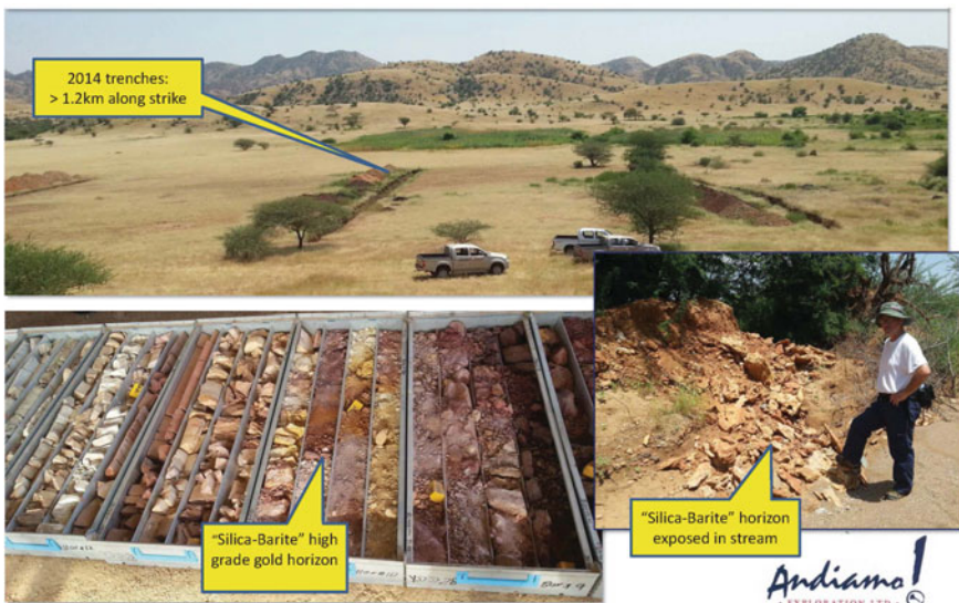
Fig. 8.41 Field photographs showing the site of trench sampling, oxidized silica-barite exposure, and core samples of the Yacob Dewar gold mine, Eritrea. (Source Andiamo Exploration Ltd)
