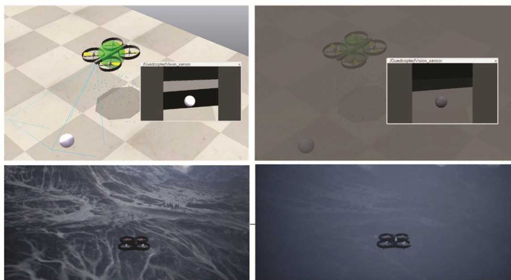
Figure 17. Top two figures show the effect of sun azimuth angle and fog affecting vision sensor capabilities. The bottom two figures show a UAV flying in clear weather ( left ) and in fog and snow weather ( right ) using Microsoft AirSim.
