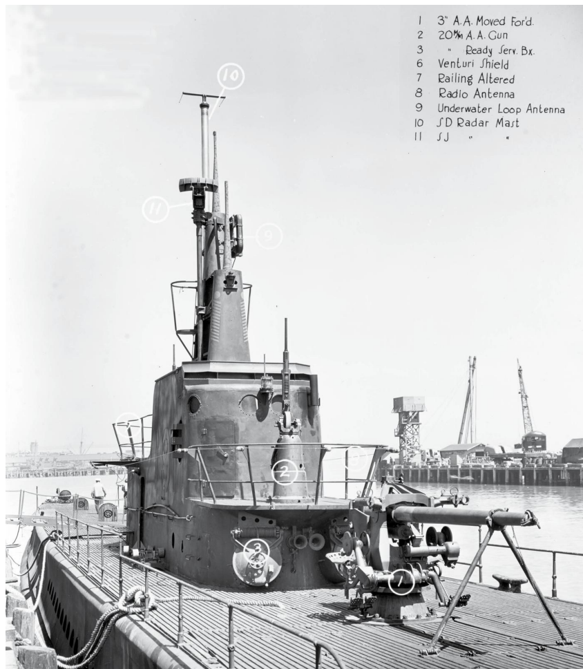
A fleet submarine's radars were mounted on its radar mast, behind the night periscope. The SJ surface search radar's antenna is at the top of the mast (10) and the SD air search radar's antenna is the grid arc beneath the SJ antenna (11). (USNHHHC)
