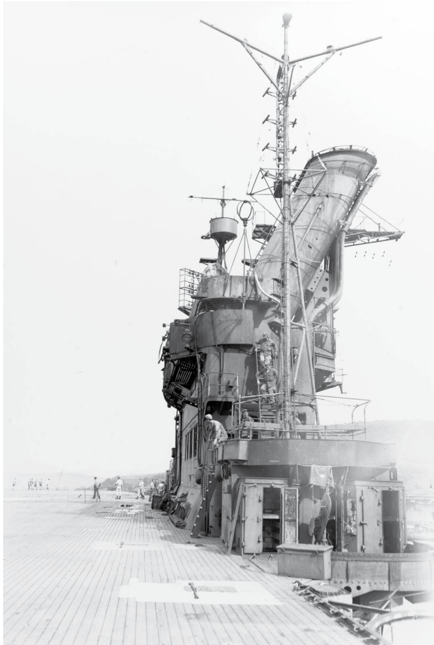
The IJN lagged behind in radar development, although by 1943 most of its carriers had radar. The Yagi antennae of Jun'yō 's Type 13 radar can be seen here on the carrier's after mast. Its Type 21 "mattress" is visible at the front of the island. (USNHHC)
