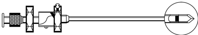
Figure 4.2 Abrams needle. Consists of two concentric tubes. The outer tube has a trocar point with a notch/window, which can be opened or closed by rotating the inner tube. A syringe can be loaded onto the end of the needle for aspiration.
