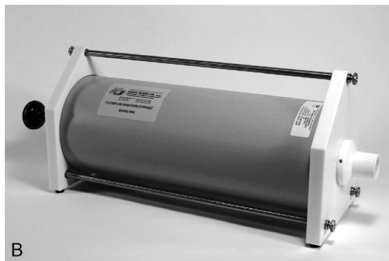
FIG. 12.1 Calibration syringes. (A) Standard 3-L syringe is used for calibration of spirometers for testing of adults and adolescents. Smaller-calibration syringes may be used for calibration and verification of pulmonary function equipment used for small children and infants. (B) A 7-L syringe. (Courtesy Hans Rudolph, Inc., Shawnee, KS.)
