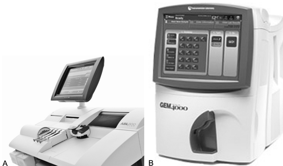
FIG. 11.30 Automated blood gas analyzer, including spectrophotometric oximeter. These systems provide automatic sample handling, flushing, and calibration. Results of sample analysis and calibrations are displayed using an integrated computer and display terminal. pH, \text{PCO}_2 , and \text{PO}_2 are measured; \text{HCO}_3^- , total \text{CO}_2 , standard bicarbonate, and other variables are calculated. This system also incorporates a spectrophotometric oximeter for analysis of Hb, \text{O}_2\text{Hb} , \text{COHb} , and \text{MetHb} . Base excess is calculated with \text{HCO}_3^- , calculated from the blood gas analysis and Hb measured by the oximeter. Additional parameters can include bilirubin, electrolytes, glucose, and lactate. (A, ABL800, courtesy Radiometer America, Westlake, OH. B, GEM, courtesy Instrumentation Laboratories, Bedford, MA. C, Siemens Rapid Lab, courtesy Siemens Healthcare, Tarrytown, NY.)
