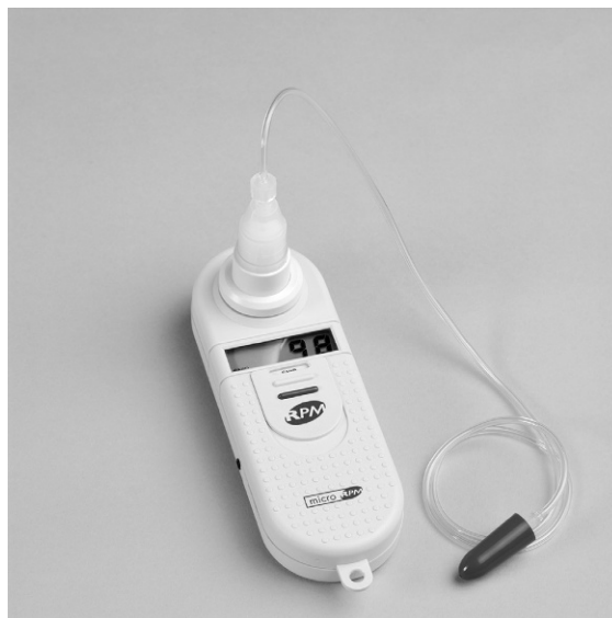
FIG. 10.4 Handheld device for measuring sniff nasal inspiratory pressure (SNIP). (Courtesy Vyair Medical, Mettawa, IL.)
