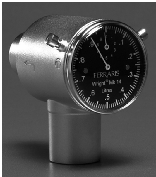
FIG. 11.5 Turbine-type flow sensor. The Wright Mk14 respirometer is shown. A rotating vane mounted on jeweled bearings drives reduction gears connected to the main dial.
