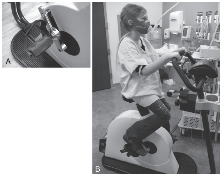
FIG. 8.27 (A) An adjustable pedal crankshaft used to test smaller patients when performing cardiopulmonary exercise tests (CPETs). (B) An 8-year-old female positioned on a cycle ergometer with a facemask interfaced with a pneumotachometer to measure exhaled air.
