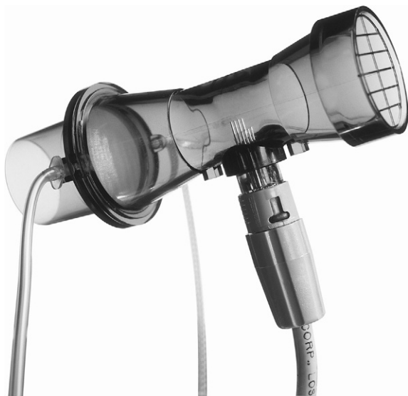
FIG. 11.9 Heated-wire flow sensor. A flow tube contains very thin, paired stainless steel wires. The wires are maintained at two temperatures exceeding body temperature and are connected by a Wheatstone bridge. The tube streamlines gas flow into laminar flow. The temperature of the wires decreases in proportion to the mass of the gas and its flow. Two wires are used; one measures expiratory flow, and the other serves as a reference. (Courtesy Vyair, Mettawa, IL.)
