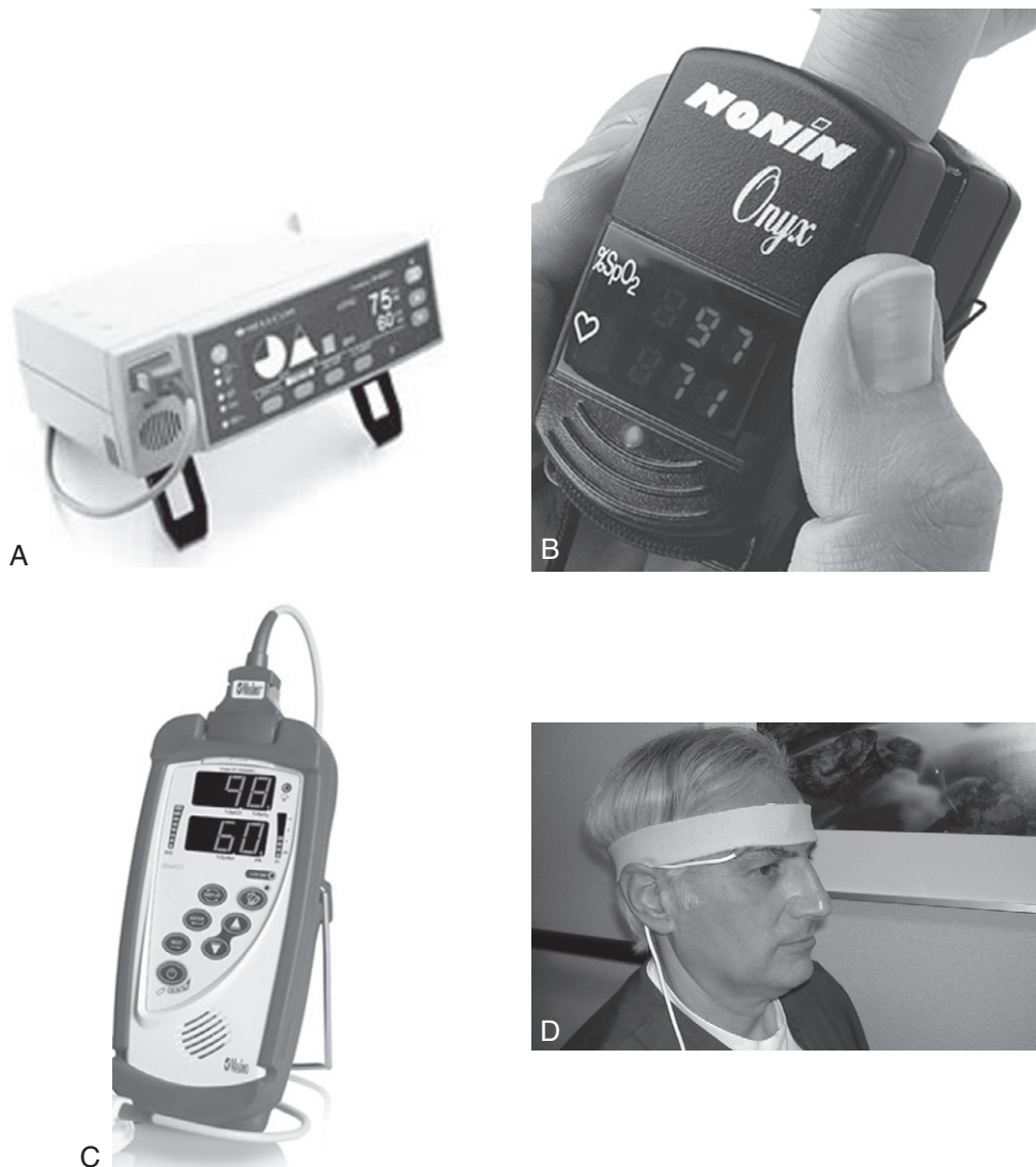
FIG. 11.34 Pulse oximeters. Most pulse oximeters provide a digital display of oxygen saturation and pulse rate. (A) Desktop unit. (B) A small, portable pulse oximeter that fits over the patient's finger. Miniaturized components allow a device of this size to be easily transported. (C) A sophisticated multiwavelength pulse oximeter that is capable of measuring Hgb, COHb, and MetHb, in addition to O_2 Hb and pulse rate. (D) Reflectance pulse oximetry probe placed on a subject's forehead. (A and D, courtesy Nellcor, a Covidien brand, Mansfield, MA. B, Courtesy Nonin Medical, Inc., Plymouth, MN. C, Courtesy Masimo Corporation, Irvine, CA.)
