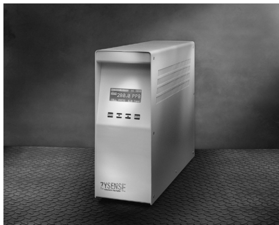
FIG. 11.25 A chemiluminescent gas analyzer for nitric oxide (NO). A commercially available analyzer designed to measure trace amounts of NO in the exhaled breath. The monitor includes an NO scrubbing device so that the subject can inhale NO-free gas and immediately exhale into the sampler. The analyzer uses the chemiluminescence effect to measure NO (see text). (Courtesy Dr. Rengarajan Ramesh, Zysense LLC, Waxhaw, NC.)
