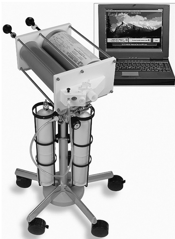
FIG. 12.3 DLCO simulator. A DLCO simulator that incorporates two large-volume syringes and multiple precision gas mixtures provides quality control for DLCO systems. The simulator attaches to the patient port of the DLCO system. (Courtesy Hans Rudolph, Inc., Kansas City, MO.)
