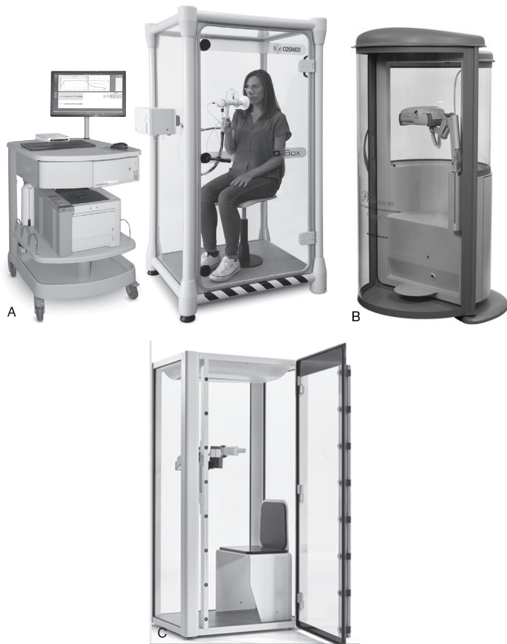
FIG. 11.16 Body plethysmograph. Examples of modern plethysmographs, with a highly transparent box, self-contained calibration equipment, and computerized data reduction and display. (A) Cosmed Q-Box. (B) MGC Platinum Elite. (C) Vyair Wheelchair box. (A, Q-Box, courtesy Cosmed, Concord, CA. B, Platinum Elite, courtesy MGC Diagnostics, St. Paul, MN. C, Vyair Wheelchair box, with permission from Vyair, Mettawa, IL.)
