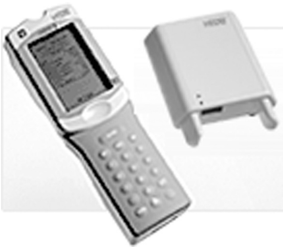
FIG. 11.31 Point-of-care (POC) blood gas analyzer. This handheld POC blood gas analyzer uses microelectrodes. It is battery powered, so it can be used in a variety of clinical settings. (Courtesy i-Stat Corp., East Windsor, NJ.)
