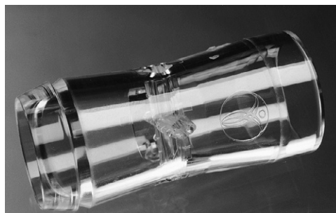
FIG. 11.10 Pitot tube flow sensor. A series of small tubes is mounted on struts in the flow tube. The tubes are connected to very sensitive pressure transducers (not shown). Using a series of transducers allows a wide range of flows to be accurately measured. Pitot tubes are mounted with struts facing both directions so that inspiratory and expiratory flow can be detected. (Courtesy MGC Diagnostics, St. Paul, MN.)
