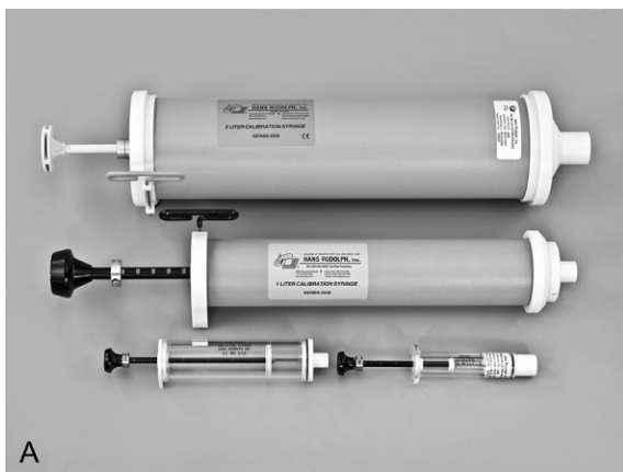
FIG. 12.1 Calibration syringes. (A) Standard 3-L syringe is used for calibration of spirometers for testing of adults and adolescents. Smaller-calibration syringes may be used for calibration and verification of pulmonary function equipment used for small children and infants. (B) A 7-L syringe. (Courtesy Hans Rudolph, Inc., Shawnee, KS.)
