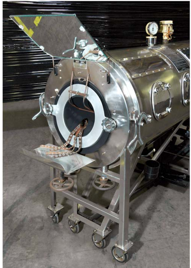
FIGURE 12.8 Emerson respirator, also known as an iron lung, which was used by polio patients whose ability to breathe was paralyzed due to this crippling viral disease. The chamber is used to create a negative pressure around the thoracic cavity, thereby, causing air to rush into the lungs. (CDC/PHIL image 6529, content providers CDC/GHO/ Mary Hilpertshauer).
