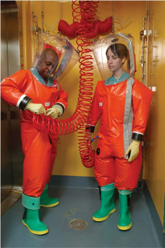
FIGURE 24.4 Centers for Disease Control microbiologists in the process of suiting up in order to access the interior of the organization's Biosafety Level-4 (BSL-4) laboratory. The scientist on the left is attaching his supportive air hose, which provides a supply of filtered, breathable air. Source: CDC Public Health Image Library ID# 10723. Content providers CDC/Dr. Scott Smith.
