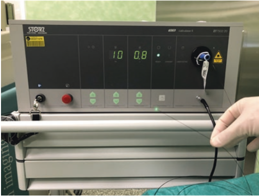
Fig. 7.1 Laser light source generator delivers cool light to the endoscope by a fine fiber-optic cable
