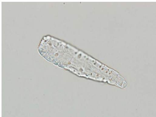
FIG. 7 An absorbent fiber (diaper or hygiene product). Note its flat appearance with perforations and its strong refractility. Brightfield.
