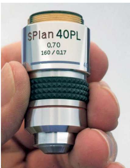
FIG. 18.6 Engravings on this objective indicate that it is a plan achromat lens (SPlan); the initial magnification is \times 40 ; the numerical aperture is 0.70; the objective is designed for a microscope with an optical tube length of 160 mm; and the coverslip thickness should be 0.17 \pm 0.01 mm.
