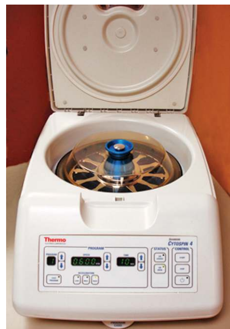
FIG. 17.2 Thermo-Scientific Cytospin 4 cyto centrifuge. (Thermo Fisher Scientific Inc., Waltham, MA.)
