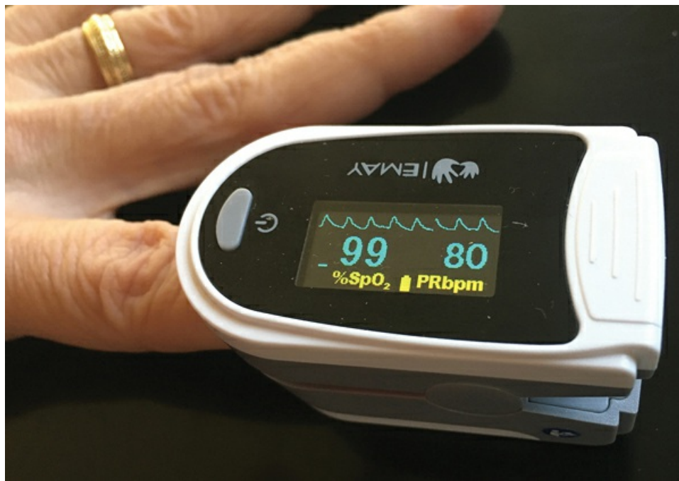
FIGURE 3.24 Pulse oximeter. The two numbers shown on the digital display represent the oxygen saturation and the heart rate.
