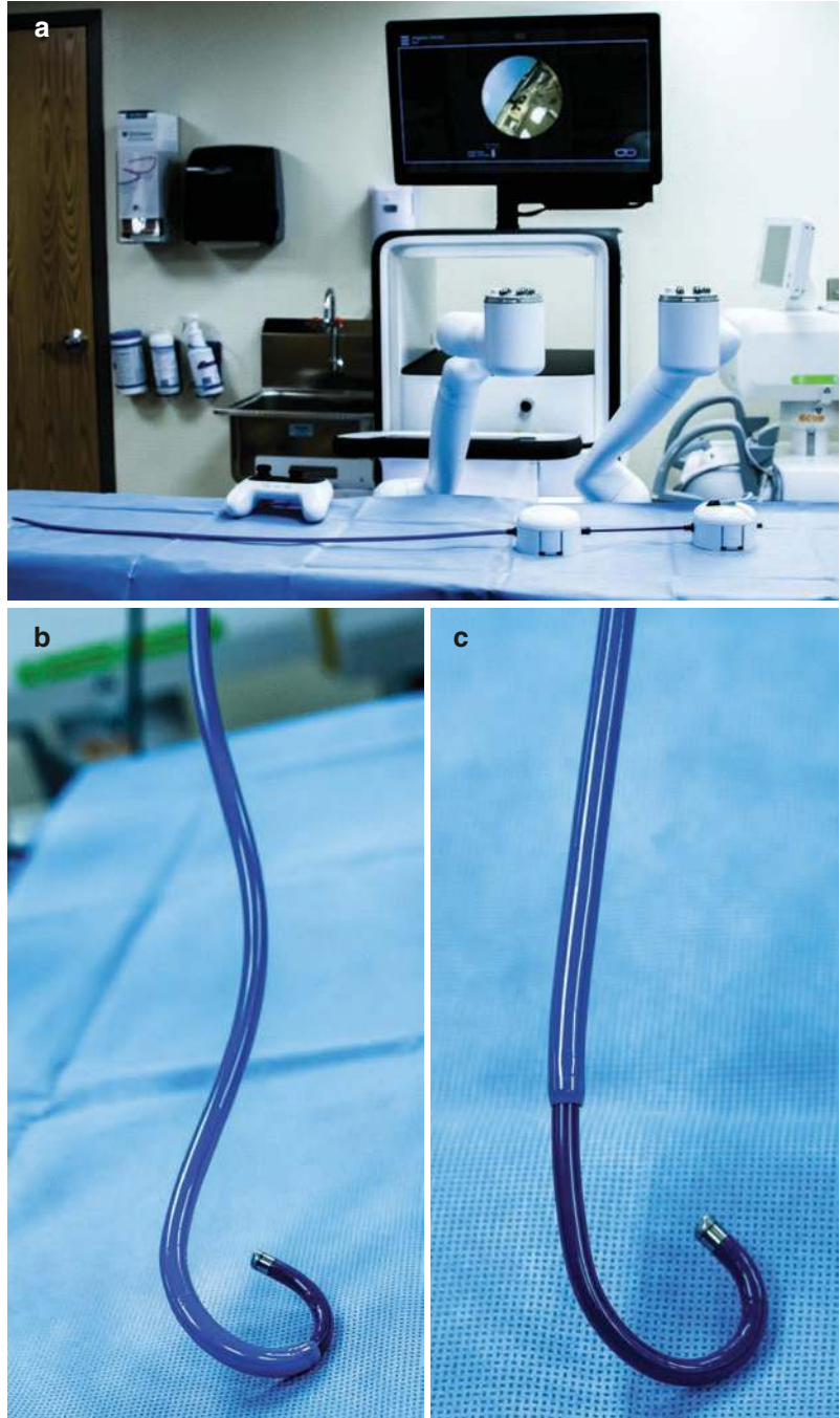
Fig. 26.3 (a) The Monarch Bronchoscope. Photograph by Leslie Kumpf RRT, CPFT. (b) The Monarch Bronchoscope in articulation. Photograph by Leslie Kumpf RRT, CPFT. (c) The inner bronchoscope of the Monarch platform with the bronchoscope extending beyond the outer sheath. Photograph by Leslie Kumpf RRT, CPFT
