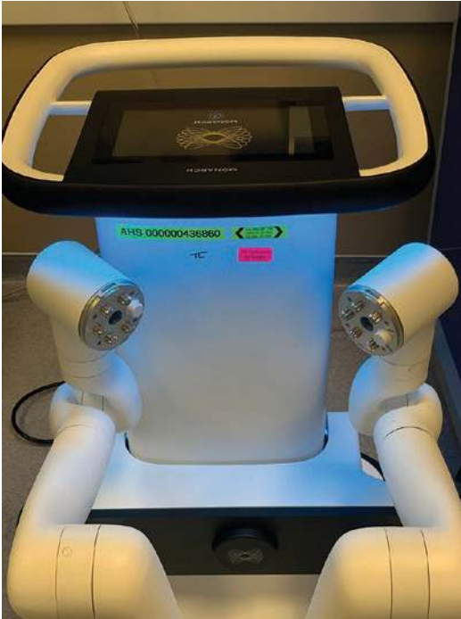
Fig. 26.4 The robotic arms of the Monarch platform
