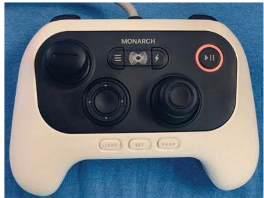
Fig. 26.7 The video-game based controller of the Monarch platform
