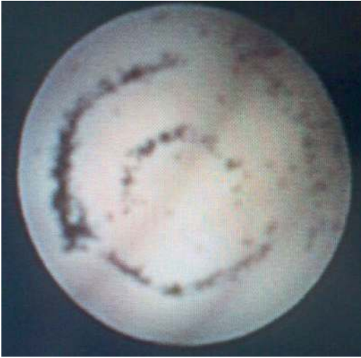
Fig. 3.3 Black dots corresponding to broken fibers after the ultrathin fibrobronchoscope was accidentally bitten by a patient
