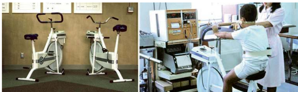
Fig. 6.63 Bicycle ergometer. Left: The height of the saddle was lowered to analyze the expired gas during exercise in elementary school students with a height of around 120 cm
