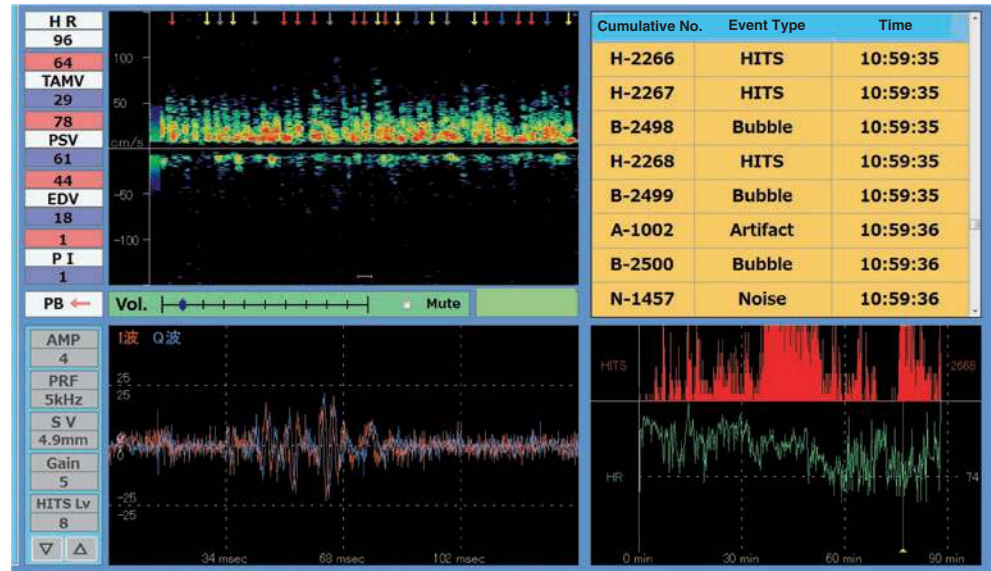
Fig. 5.4 Confirmation monitor screen in FURUHATA. The red dots in the upper left figure are events such as bubbles were observed. The lower right red graph shows the number of measurements per minute over time. By placing the yellow cursor on the time axis, the eight samples measured before and after that time will be identified as bubble, HITS, Noise, or Artifact, and displayed in the upper right figure. The accuracy of each measured event can be reconfirmed in the frequency waveform (lower left figure). HITS: High Intensity Transient Signal
