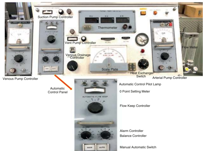
Fig. 2.9 Control panel of DV-3D heart-lung machine. With automatic pump rotation control
