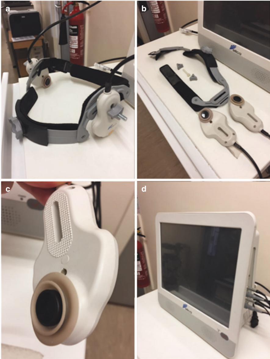
Fig. 65.1 Delica EMS 9D rTCD System. rTCD robotic transcranial Doppler. Panel (a) – Adjustable headband with ratchet system. Bilateral TCD probe/robotic construct attached. Panel (b) – Demonstrates ability to completely dismantle headband system, enabling reassembly around a patient’s head. Panel (c) – TCD probe and robotic drive construct. Black 1–2 MHz TCD probe is surrounded by optional rubber ring, designed to retain ultrasound gel and reduced gel drying. Panel (d) – Delica EMS 9D rTCD monitor
