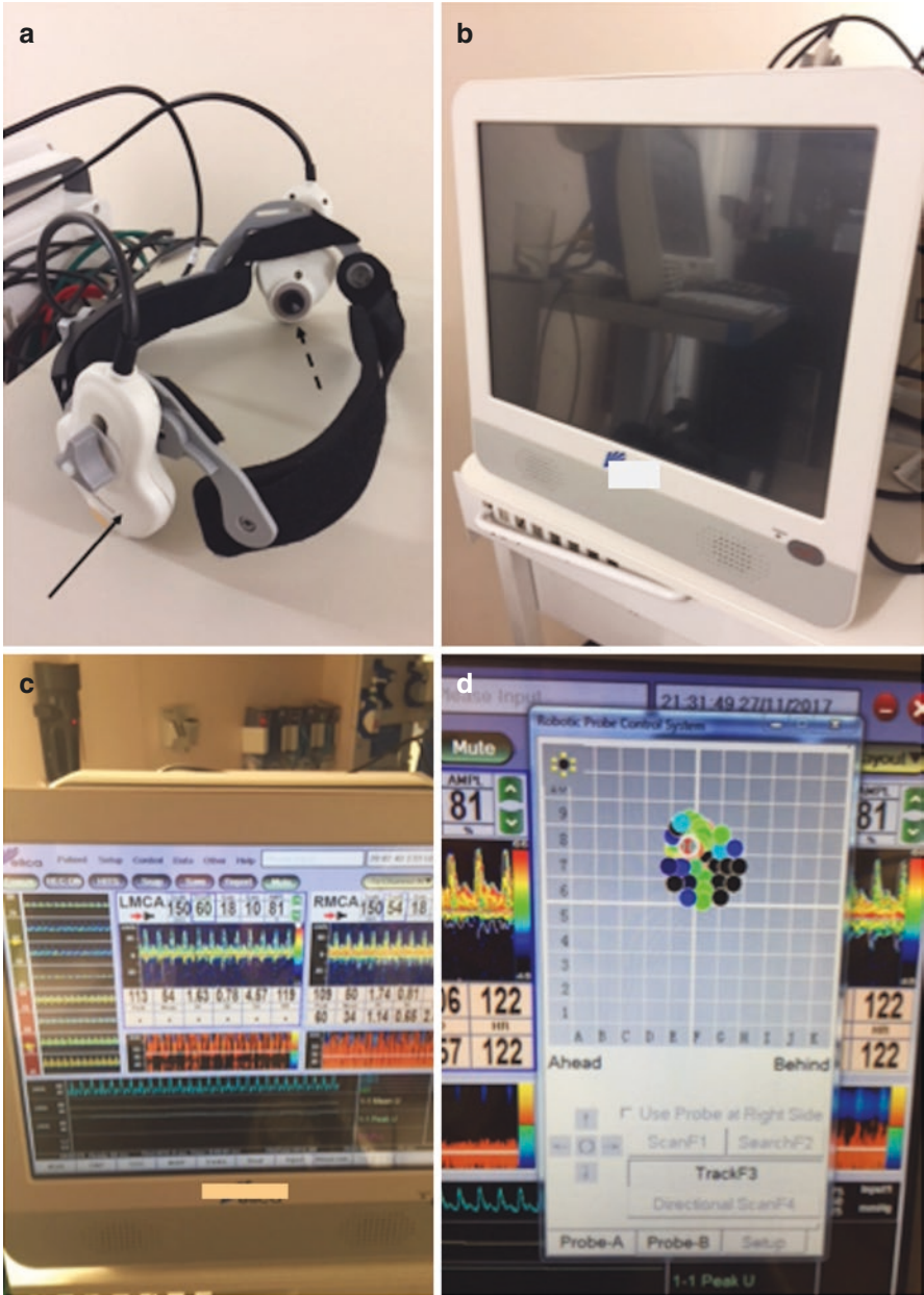
Fig. 23.3 New robotic TCD system TCD = transcranial Doppler. Panel (a): Head band holder for bilateral robotic controlled TCD probes. Solid black arrow denotes the encased robotic control system. Dashed arrow indicates black TCD probe, which is automatically moved by robotic device in response to automated signal detection algorithm. Panel (b): Robotic TCD touch-screen monitor. Panel (c): Bilateral TCD recording in real time. Panel (d): Robotic TCD probed controlling system displaying various probes positions insonated automatically via robotic system, with color-coded intensities
