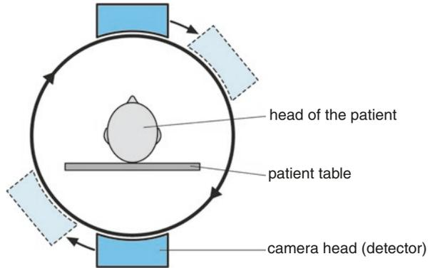
**Fig. 2.3** Principle of PET: In PET, simultaneous events, so-called coincidences, are measured. This enables the exact spatial assignment of a signal. (Adapted from Otte (2001b))
