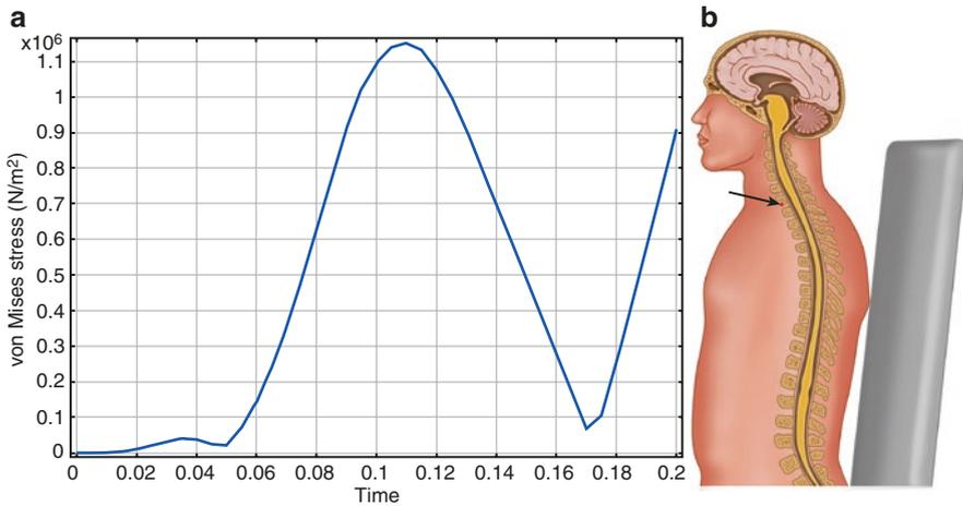
**Fig. 1.8** (a) FEM simulation of the predicted maximum von Mises stress in the C6-C7 disc during whiplash with 200 ms acceleration/deceleration duration (without headrests) according to the study setting of Teo et al. (2005), von Mises stress in  $\text{N/m}^2 \cdot 10^6$ , time in s; (b) The measurement point in our FEM simulation model, see the red point indicated by the arrow
