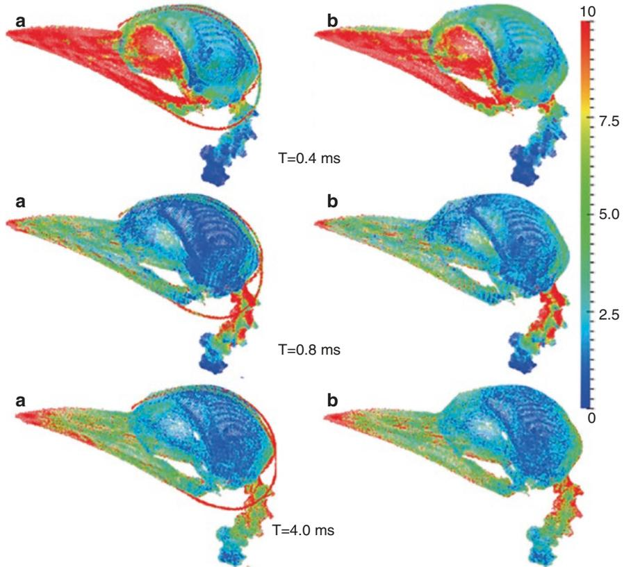
**Fig. 1.12** von Mises stress contours of the woodpecker endoskeleton at different time points under 1 m/s impact velocity, color bar in  $10^5$  Pa; (a) model with the help of the hyoid bone, (b) model without the help of the hyoid bone. (Copyright 2015 by Liu et al., doi:<https://doi.org/10.1371/journal.pone.0122677>. Published by PLoS One under the terms of the Creative Commons Attribution License CC BY 4.0, which permits unrestricted use, distribution, and reproduction in any medium)
