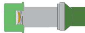
Cross section of Port Protector demonstrating how the alcohol sponge passively disinfects the surface of a Needle Free Connector
