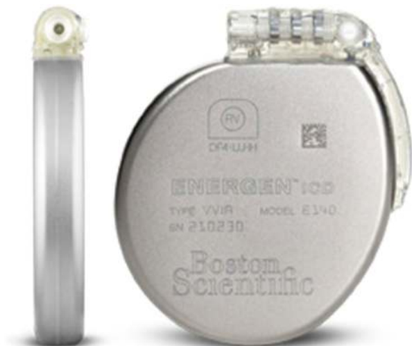
Fig. 7.3 An implantable cardioverter defibrillator (ICD) pulse generator. This device is connected to at least one wire, which is typically inserted through a blood vessel into the heart. Your doctor may prescribe an ICD if you are at risk for sudden cardiac death. It helps to treat lethal arrhythmias such as ventricular tachycardia and ventricular fibrillation. Note that the specific type of ICD shown in this figure is a biventricular device (see Chap. 31). (Image provided courtesy of Boston Scientific. ©2020 Boston Scientific Corporation or its affiliates. All rights reserved)
