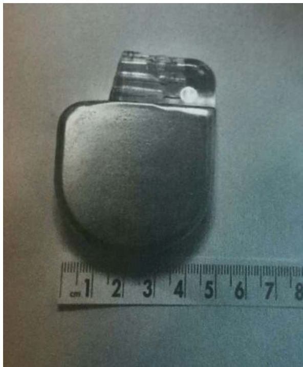
Fig. 31.1 A biventricular implantable cardioverter defibrillator (ICD) pulse generator used to treat people who have congestive heart failure and are at risk for sudden cardiac death. (Adapted from T.J. Cohen, A Patient's Guide to Heart Rhythm Problems (Baltimore, MD: The Johns Hopkins University Press, 2010), p. 115)
