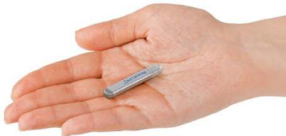
Fig. 19.3 This figure shows an injectable loop recorder (called the Revel LinQ, manufactured by Medtronic Inc.). This device can record heart rhythms remotely for up to 3 years and is useful for detecting and correlating heart rhythms with symptoms, as well as identifying atrial fibrillation in patients with a history of embolic stroke of unknown etiology. (Reproduced via permission from HMP Communications LLC and Practical Electrophysiology 3rd Edition; Reproduced with permission of Medtronic, Inc.)
