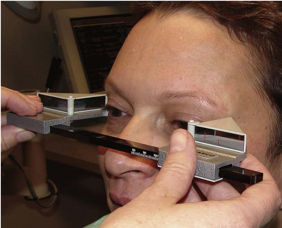
FIGURE 6.4 Hertel exophthalmometer for the measurement of proptosis.
