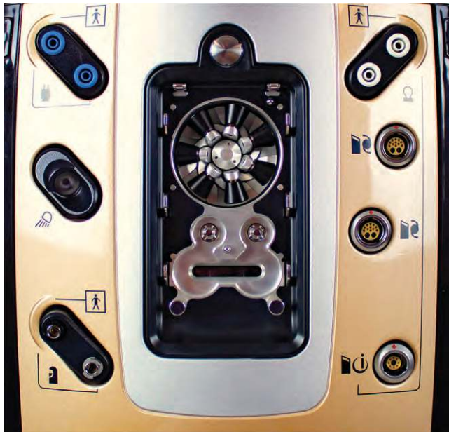
Fig. 20.7 This image of the Centurion console shows the seven rollers associated with the peristaltic pump.
