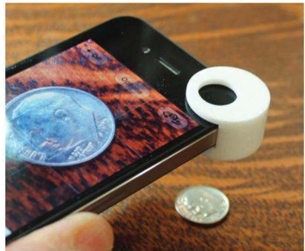
Fig. 12.125 A third-party macro lens attachment to a smart phone turns the iphone into a magnifier.
