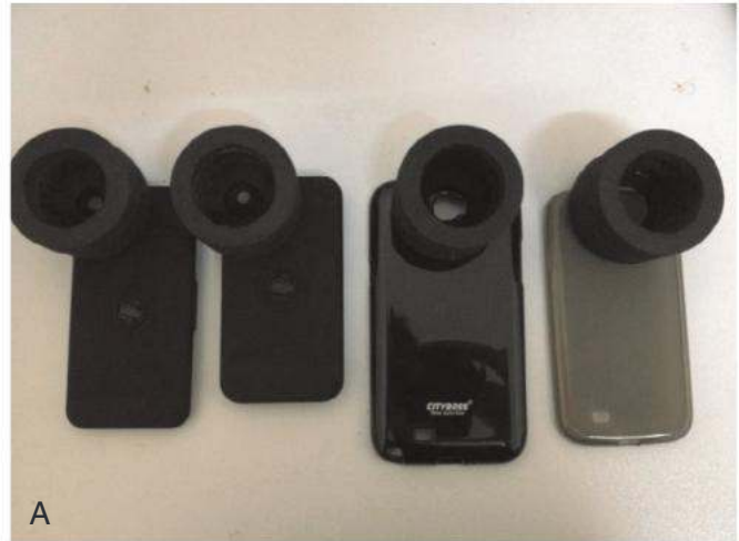
Fig. 12.125 A third-party macro lens attachment to a smart phone turns the iphone into a magnifier.
