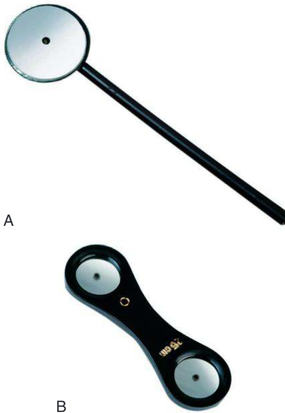
Fig. 5.12 Mirror retinoscopes: A, plane mirror; B, Priestley–Smith's mirror.
