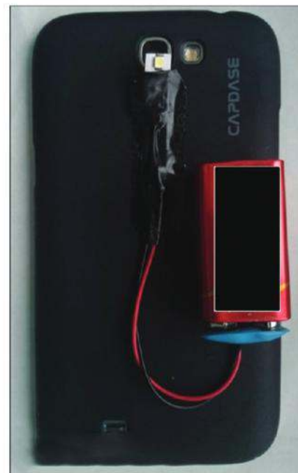
Fig. 12.132 Modification of the mobile phone camera by affixing a light emitting diode light with external power supply.
