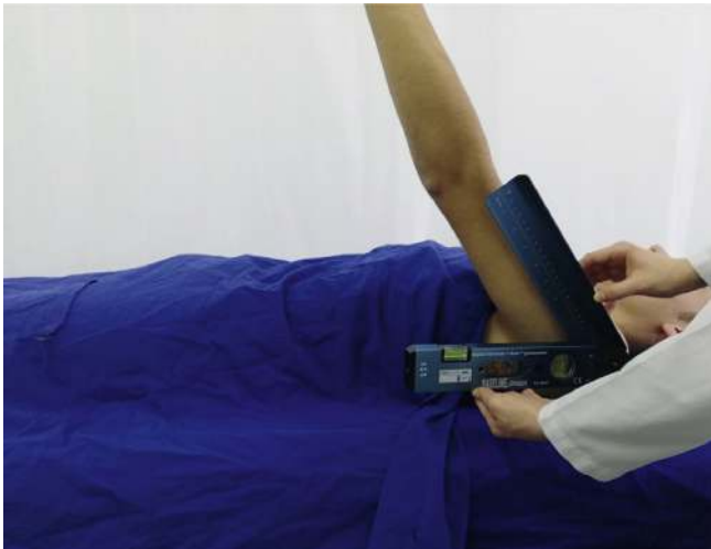
FIG. 3.25 Electronic goniometer. (From Zileli A, et al: Reliability and validity analyzes of Kinect V2 based on measurement system for shoulder motions, JJBE , 76, 2020.)
