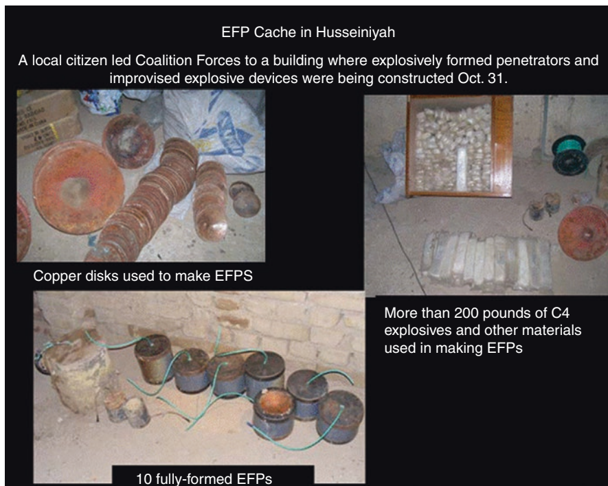
Fig. 1.3 Cache of explosively formed penetrators (EFPs) found in Iraq, 2007. (Courtesy US Department of Defense)
