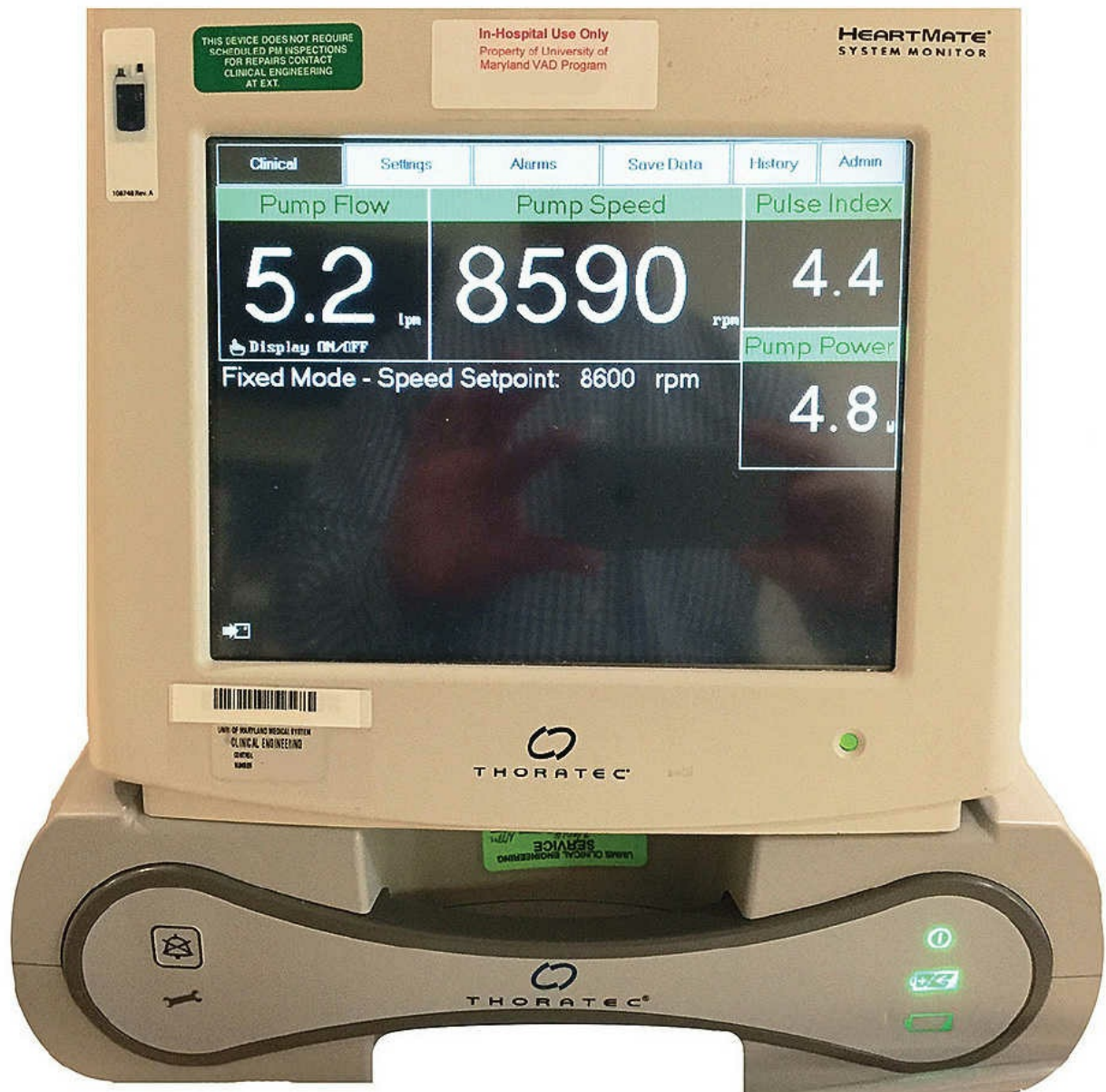
FIGURE 15-4. Thoratec HeartMate II Inpatient Console. Simultaneously displays LVAD flow, speed, power, and pulsatility index in addition to other device-specific data.
