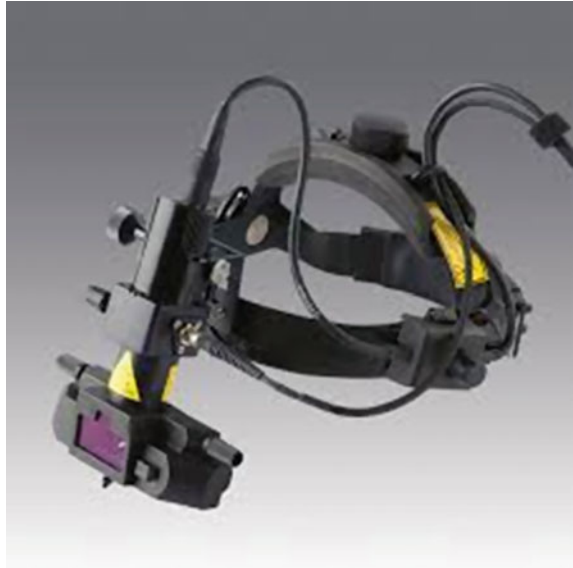
Fig. 7.2 Headset and cable for laser indirect ophthalmoscopy (Ellex, Australia). The cable is connected to a laser device
