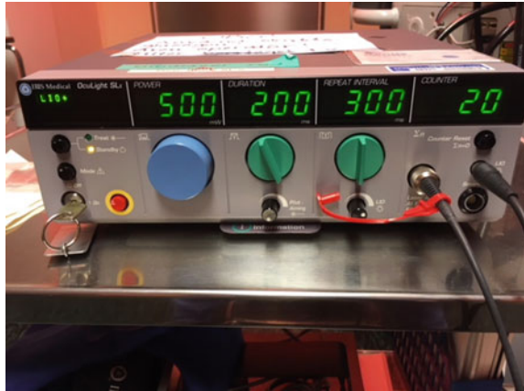
Fig. 11.2 A diode laser (Iridex) and two attached cables from binocular laser ophthalmoscope for laser and light
