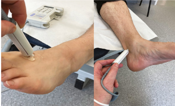
Figure 30.2 Using Doppler ultrasound in vascular assessment (shown here in an ankle/brachial pressure index assessment). Source: Courtesy of Edmonds and Foster (2005).
