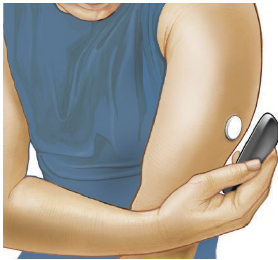
FIGURE 10.1 Freestyle Libre flash glucose monitoring system (Abbott Diabetes Care). This comprises a sensor worn on the back of the arm. A small subcutaneous filament measures interstitial blood glucose every minute and stores data every 15 minutes. The device can be scanned using a dedicated reader or smartphone. The reader shows the glucose level and trend using arrows. An ambulatory glucose profile is also produced which allows for pattern analysis. Source: FreeStyle Libre is a trademark of Abbott or its related companies. Reproduced with permission of Abbott, © 2021. All rights reserved.
