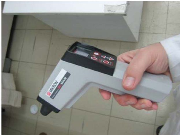
Figure 10.1 A thermometer for measuring skin temperature using infrared radiation, without touching the skin.
