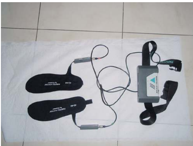
Figure 2.28 The in-shoe measurement system. This comprises insoles with attached pressure sensors that transmit the information (either wirelessly or via a wire, as in this photograph) to a central recorder of the foot pressures, usually attached to the patient's belt.
