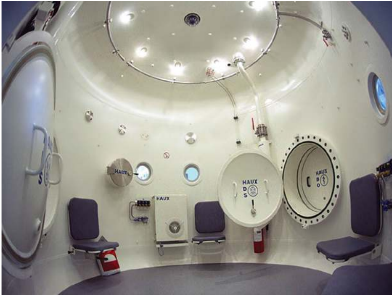
Figure 13.62 A multiplace chamber to treat multiple individuals with hyperbaric oxygen.
