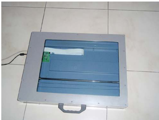
Figure 2.26 A scanner. The patient stands on the scanner surface barefoot, while the instrument scans the plantar surfaces of the feet and gives an analysis on a computer screen.
