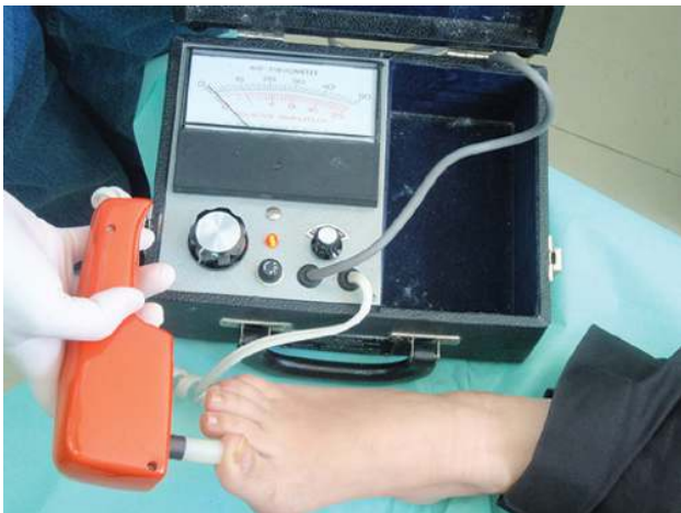
Figure 2.8 The vibration perception threshold is tested at the tip of the big toe using the biothesiometer. The patient is asked to identify when the vibration starts while the voltage of the instrument is gradually increased.
