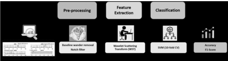
FIGURE 1.10 Block diagram of WST-based ECG arrhythmia classification framework (Nahak and Saha, 2023).
