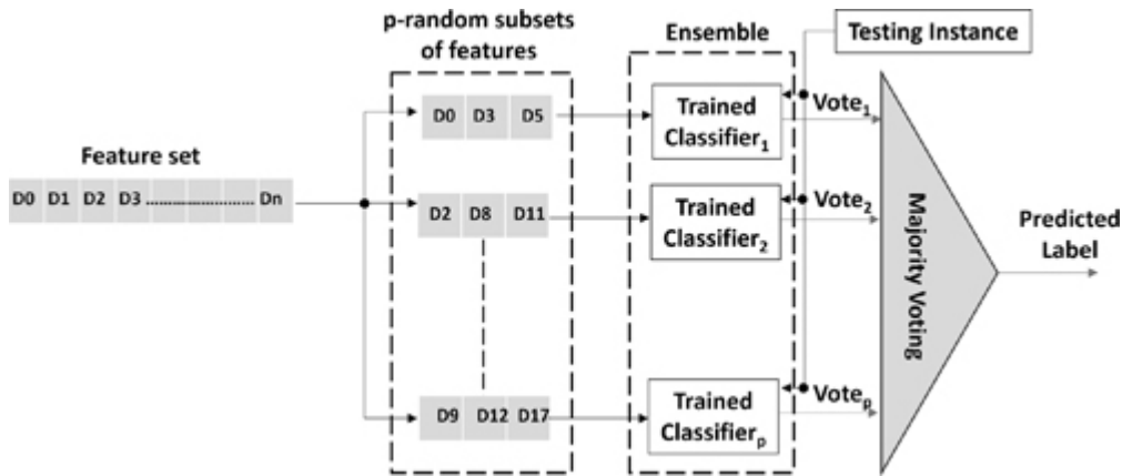
FIGURE 2.3 The principle of the Random Subspace algorithm. ↩
