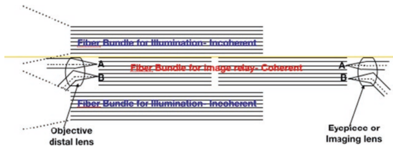
Fig. 10.4 Light and image fiber arrangement
