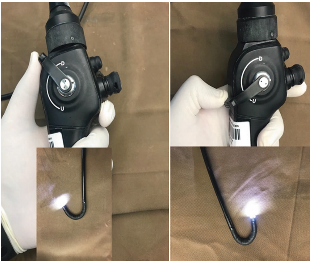
Fig. 21.2 Movements of control lever and tip of insertion cord
