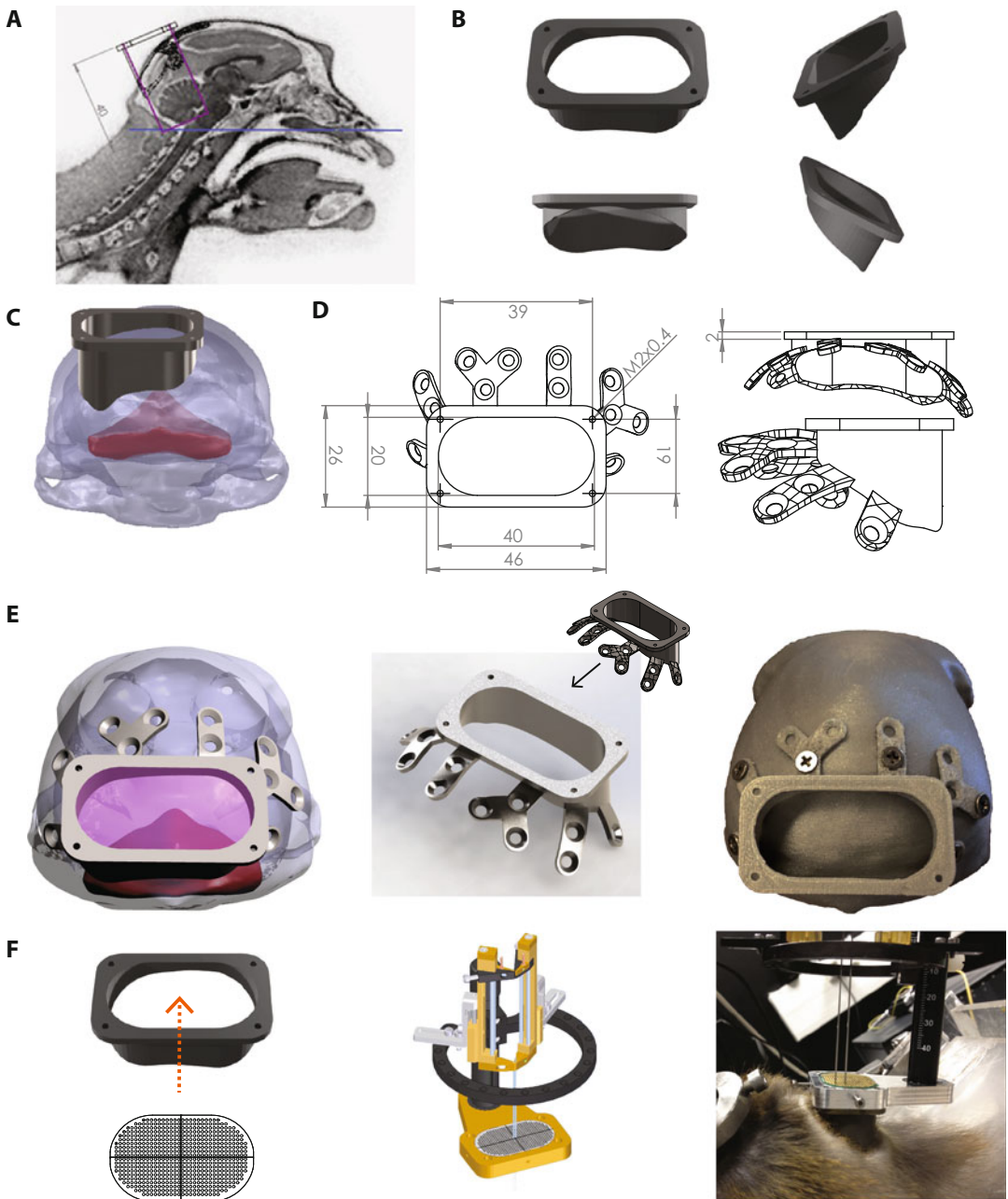
Fig. 3 Customized chamber for cerebellar recordings. (a) Chamber angle and depth plan from MRI sagittal cut. Based on the MRI, we calculated the chamber size and angle to be able to reach all vermal lobules and left lateral cerebellum. This can be easily expanded to cover the whole right cerebellum. (b) Custom cerebellar chamber rendered after shaping the bottom to the skull. (c) Posterior view of the chamber fitted on the MRI reconstructed skull (gray) and cerebellar (red) target locations. (d) Engineering drawing of the chamber with the legs to be screwed onto the skull. The legs were also skull-fitted. (e) Left Posterior view of the chamber with the legs fitted on the skull on top of the occipital bone. Middle After having completed the CAD chamber, the chamber was printed in 3D printed in Grade 5 Titanium alloy. Right Plastic 3D printed skull and chamber that facilitated surgery preparation. (f) Left Custom two-sided grid (to cover all the available recording space in the chamber) to guide electrode recordings. Every hole is 1 mm × 1 mm apart. Middle Custom grid mounted
