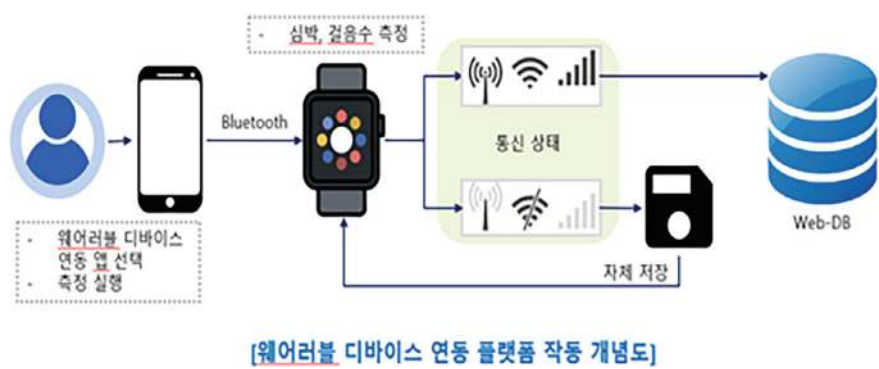
Fig.6 Method of storing data according to communication with wearable device linkage application
