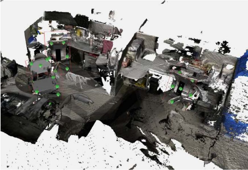
Fig. 2 Objects models aligned on the scanned point cloud
