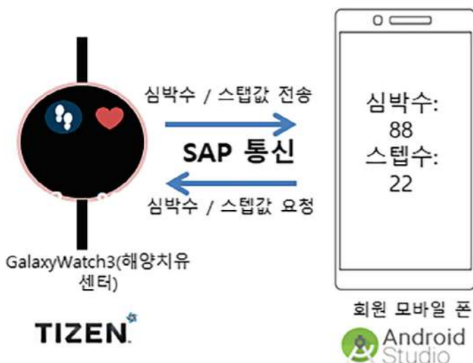
Fig. 1 Communication between wearable devices and applications using SAP communication
