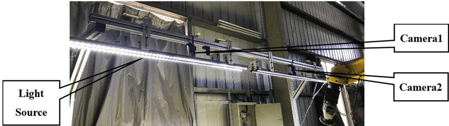
Fig. 3. Camera and light source layout.
